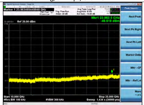
Conducted Spurious, 10-25GHz 802.11g, 54Mbps, Channel 11
