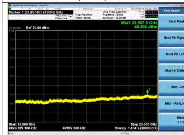
Conducted Spurious, 10-25GHz 802.11n, MCS0, Channel 1
