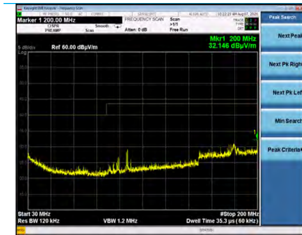
30-200 MHz, Horizontal Antenna, Vertical EUT 802.11b, 1Mbps, Channel 1
