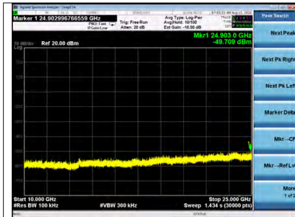
Conducted Spurious, 10-25GHz 802.11b, 1Mbps, Channel 6
