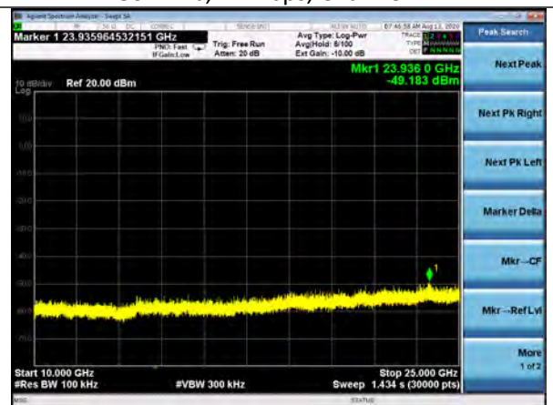
Conducted Spurious, 10-25GHz 802.11b, 11Mbps, Channel 11
