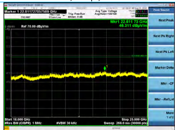
18-25 GHz, Vertical Antenna, Vertical EUT 802.11b, 1Mbps, Channel 11
