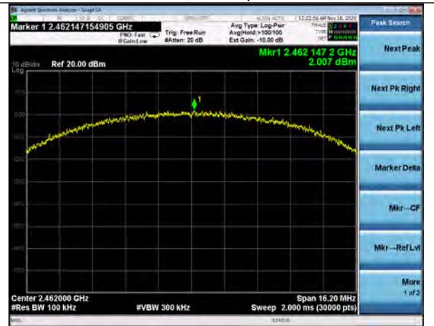
PSD, 802.11b, 11Mbps, Channel 11
