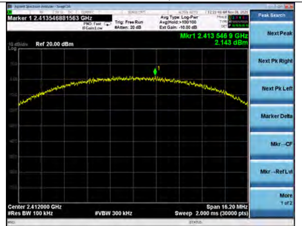
PSD, 802.11b, 11Mbps, Channel 1
