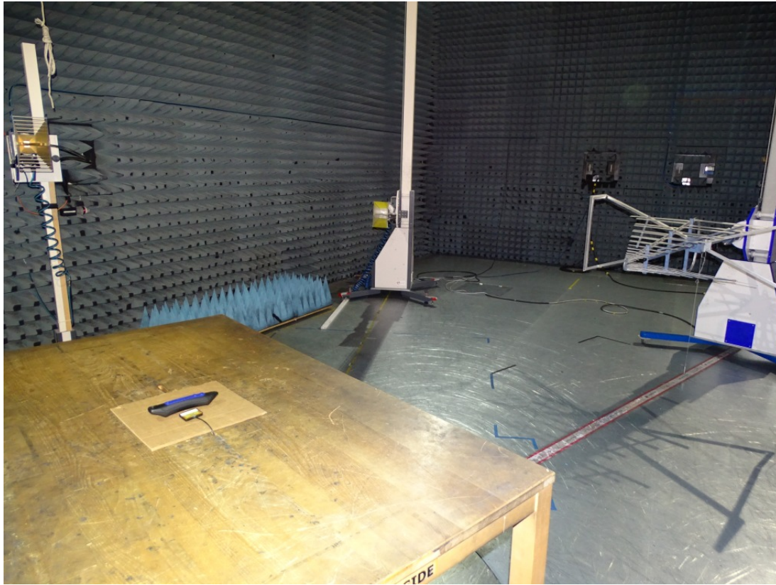
Photo 3: Test setup for radiated measurements (30 MHz – 1 GHz)
