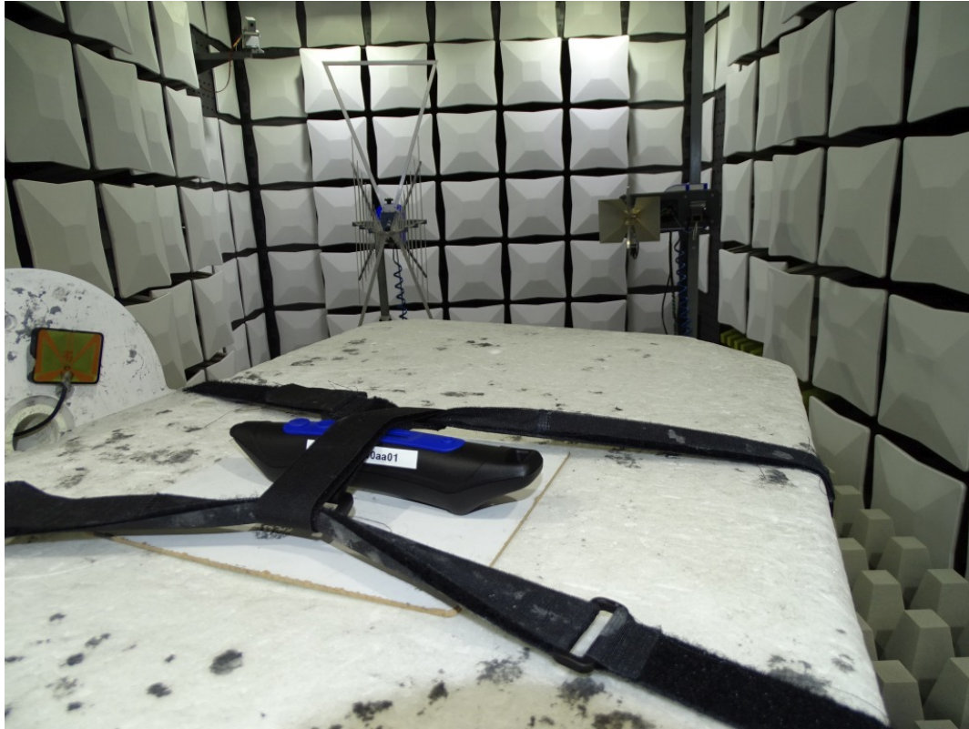
Photo 4: Test setup for radiated measurements (1 GHz – 26 GHz)
