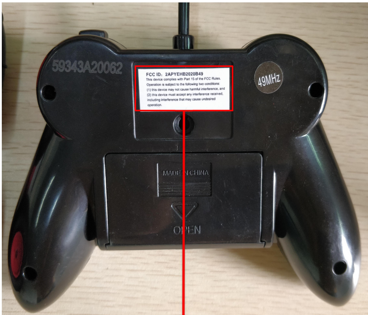
Toy RC Flip Stunt Rally 49MHz FCC ID LABEL SIZE: H 32 * W 14 MM
