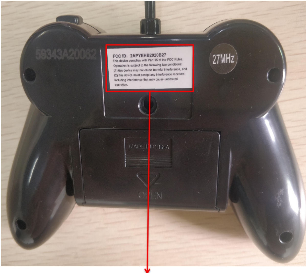
Toy RC Flip Stunt Rally 27MHz FCC ID LABEL SIZE: H 32 * W 14 MM
