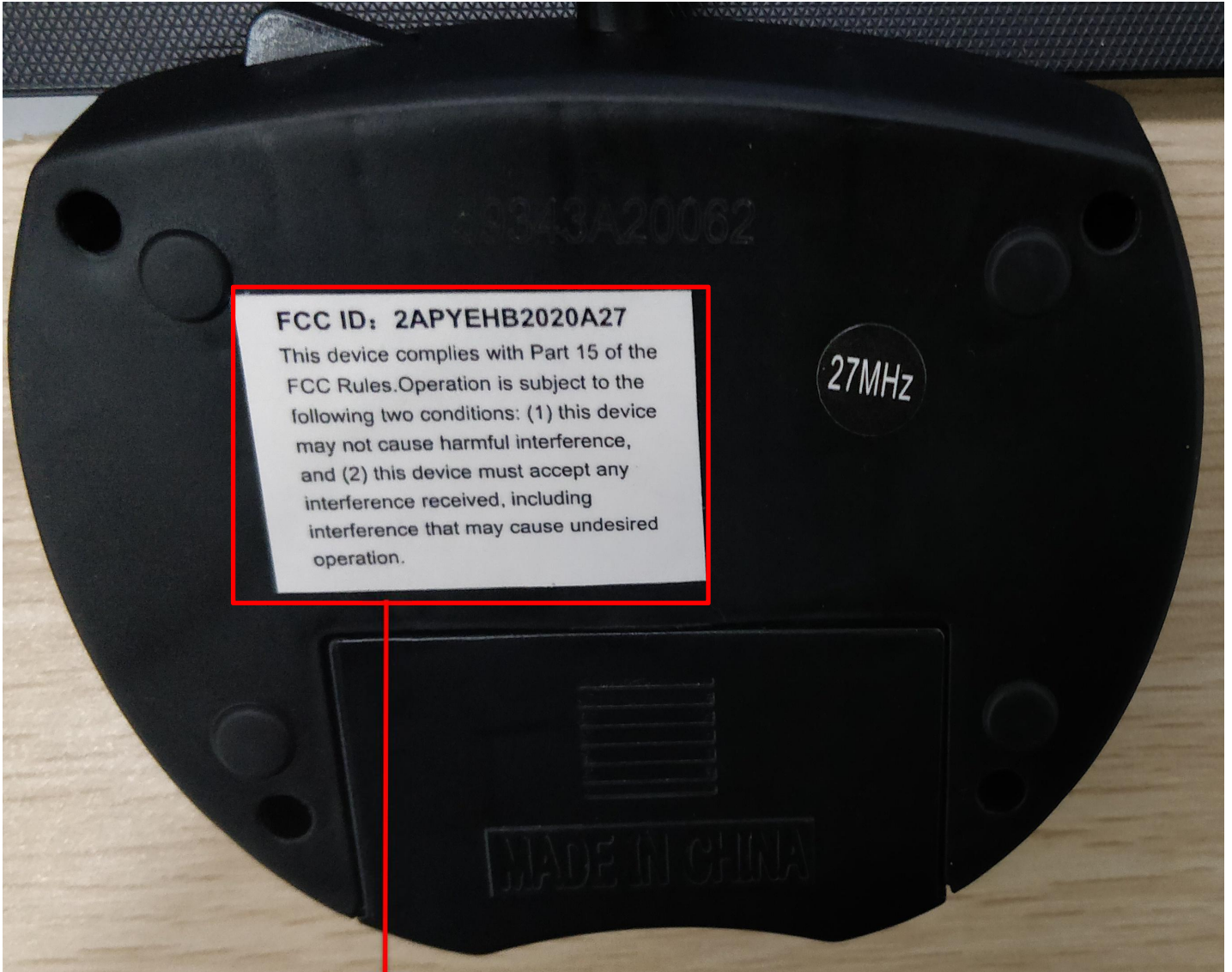
Toy RC Monster Spinning Car 27MHZ FCC ID LABEL SIZE: H 40 * W 27 MM
