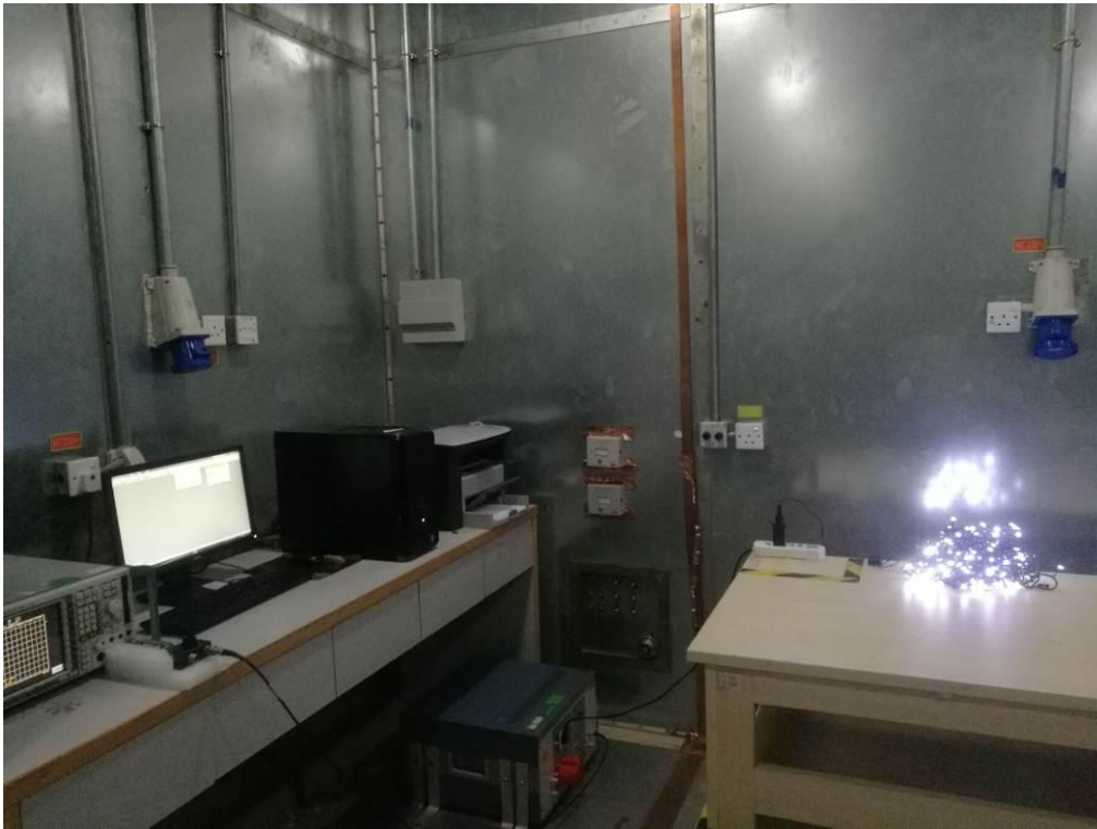
FCC RADIATED EMISSION TEST SETUP
