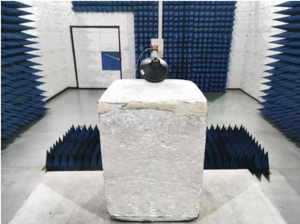
FCC RADIATED EMISSION TEST SETUP ABOVE 1GHZ
