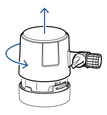
1. Turn the back of the spotlight counter-clockwise (about a 1/4 turn) and open, to reveal the battery compartment.
