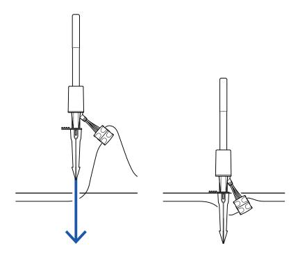
1. With the Connector attached to the low-voltage wires, position the Controller's stake where it will be installed. Loosely guide the top of the Controller with the palm of your hand. Use your foot to push down the spike and drive it into the ground.
