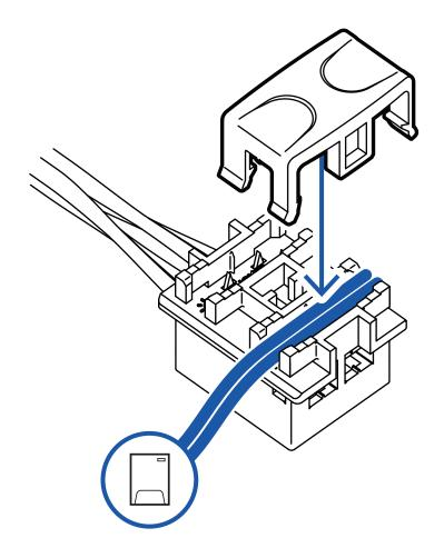
6. Replace the cap over this end of the wire, and press until the cap clips into position.
