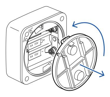
1. Press your palm against the rear plate and twist counterclockwise (about 5°) to open and access the battery compartment.
