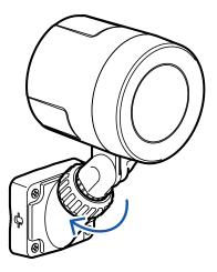
3. Set to the desired angle, and twist the locking-ring to hold the Spotlight in place.
