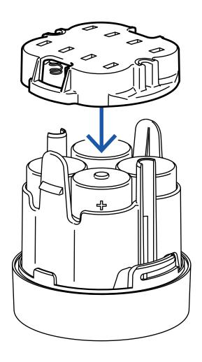
4. Replace the battery compartment cover. Press until it snaps into place.
