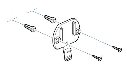
3. Fix the mount to the wall with screws. Use anchors if needed.
