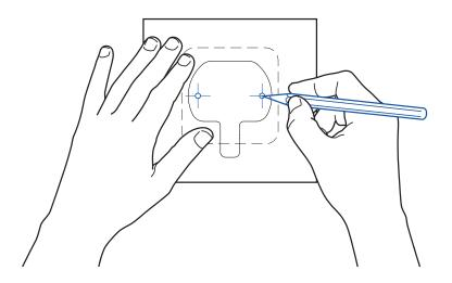
2. Use the enclosed template to mark the location where the sensor will be installed.
