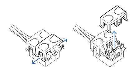
4. Remove the 2 caps from the top of the Controller's connector. Pull up on the tabs to relase the caps.
