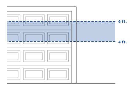
1. Choose a suitable location 4 to 6 ft. above the ground, where you'd like the sensor to detect motion and activate the light.
