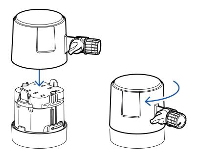
5. Replace the back of the spotlight and turn clockwise until it locks shut.
