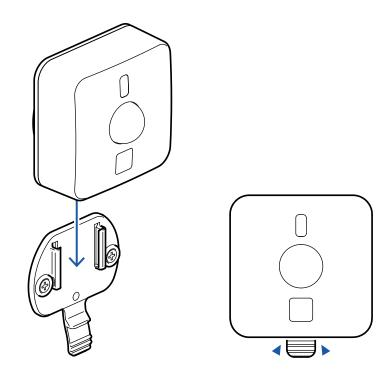
4. Slide the Motion Sensor onto the wall mount until it clicks in place.
