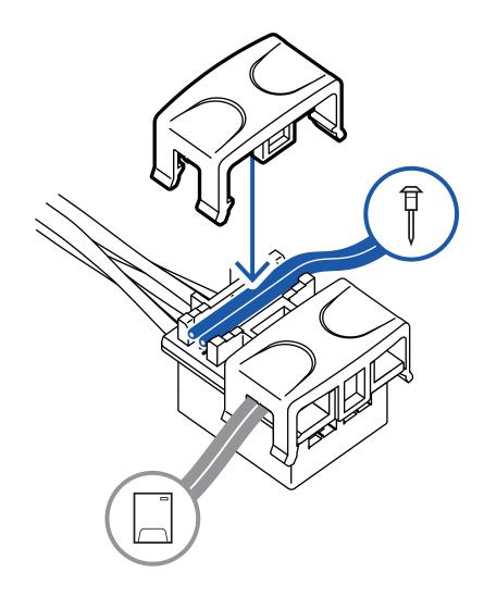
8. Align the second cap and press it into position until it snaps in place and is secured to the Connector.
