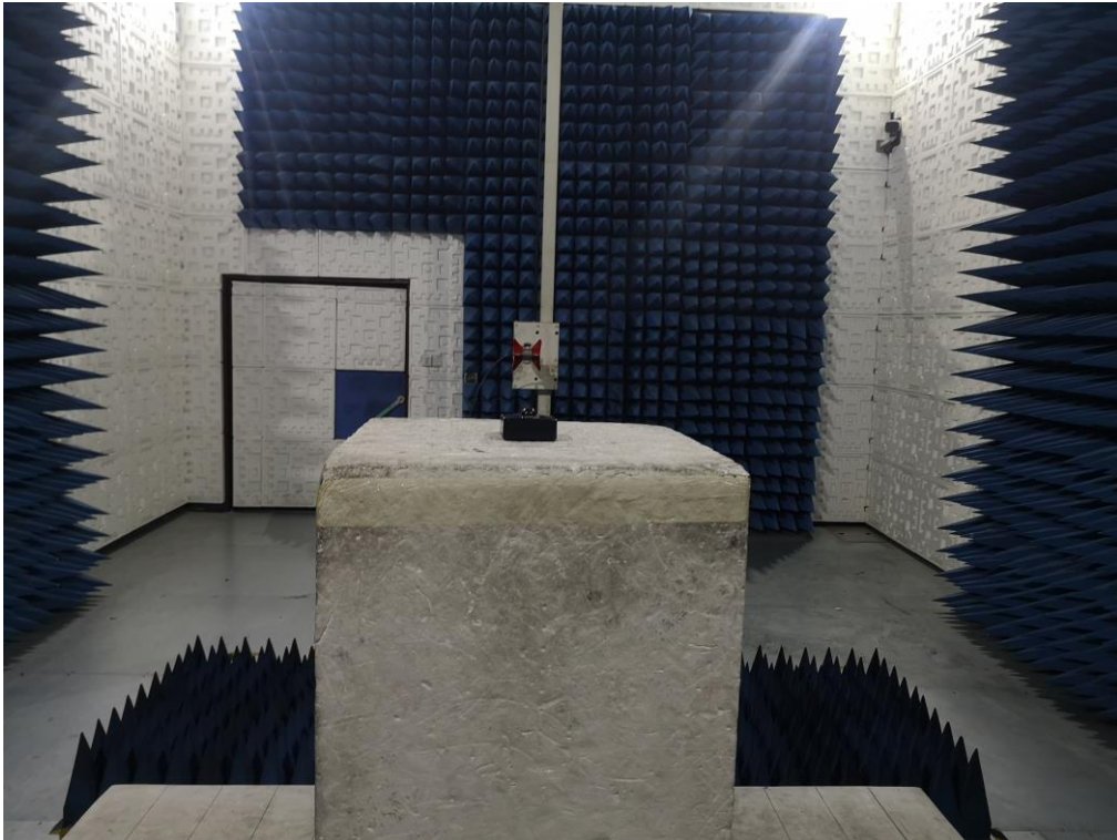
RADIATED EMISSION TEST SETUP ABOVE 1GHZ
