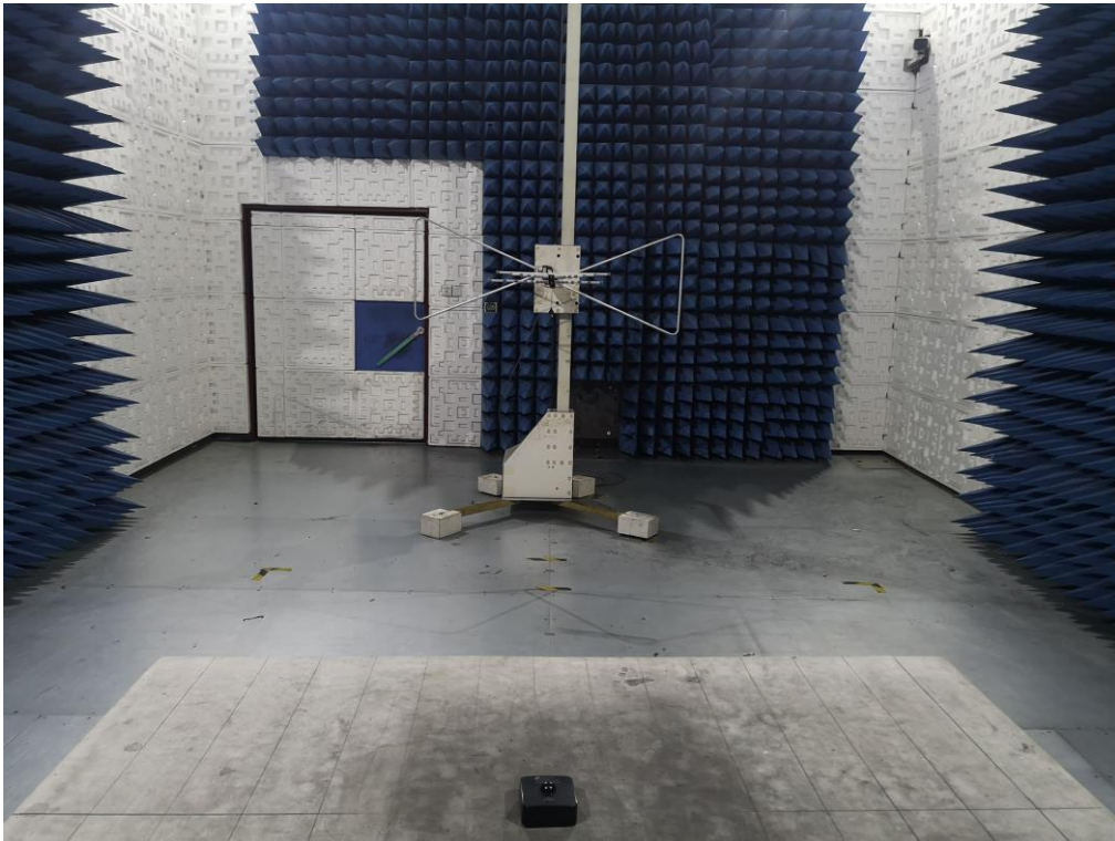
RADIATED EMISSION TEST SETUP ABOVE 1GHZ
