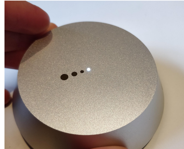
Figure 2 - Make sure that the light on top of the TTU lights up when the TTU is pressed
