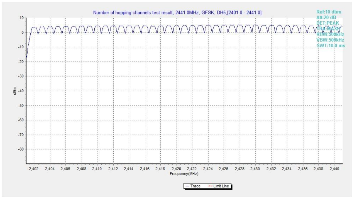
Fig.94. Number of hopping frequencies: GFSK, Channel 0 - 39
