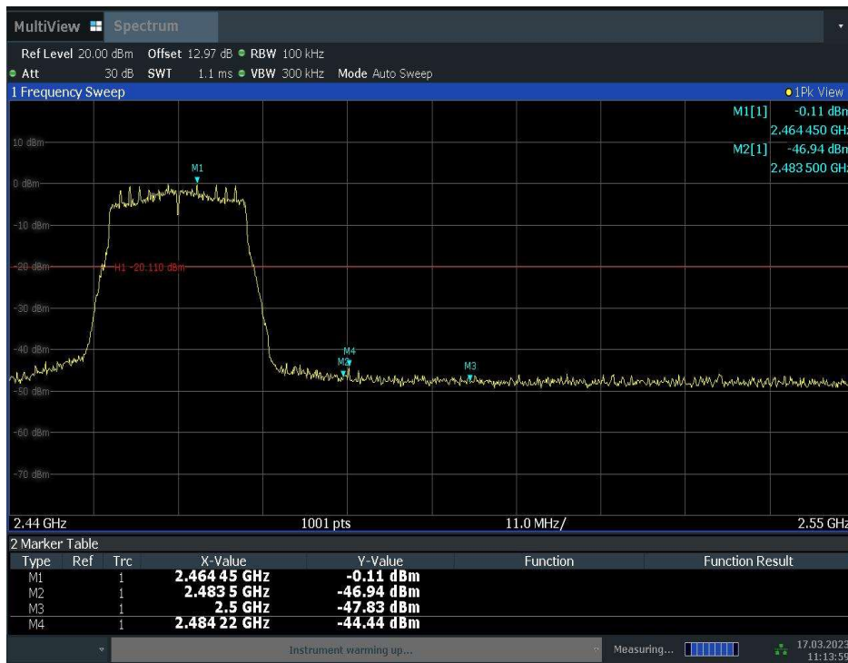
Fig.A.5.10 Band Edges (802.11n-HT20, Ch 11)
