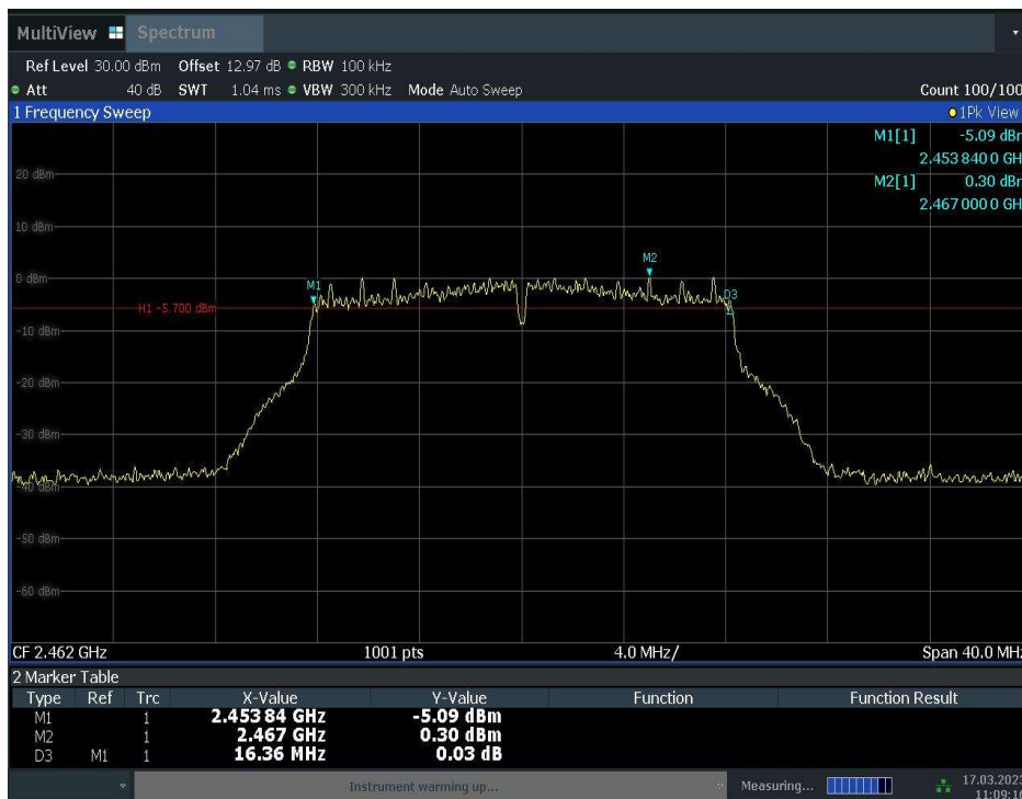
Fig.A.4.6 Occupied 6dB Bandwidth (802.11g, Ch 11)
