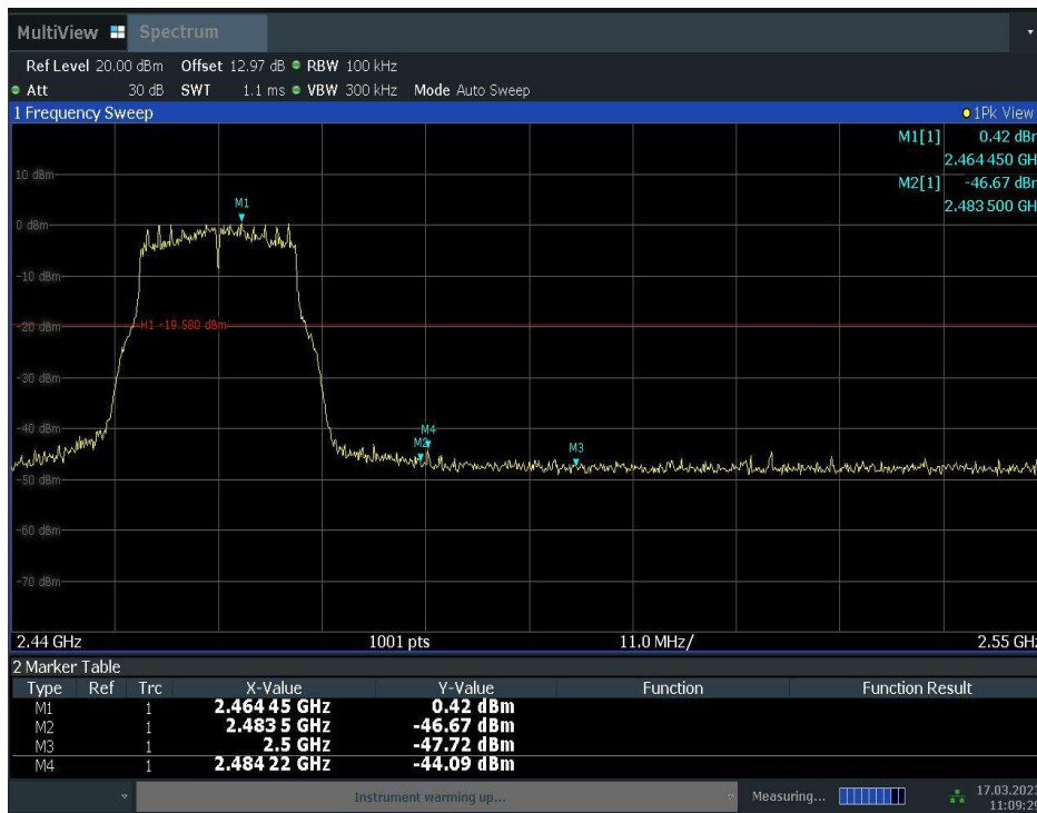
Fig.A.5.6 Band Edges (802.11g, Ch 11)
