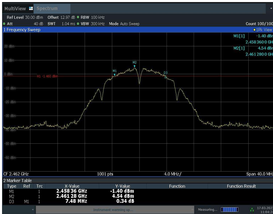
Fig.A.4.3 Occupied 6dB Bandwidth (802.11b, Ch 11)
