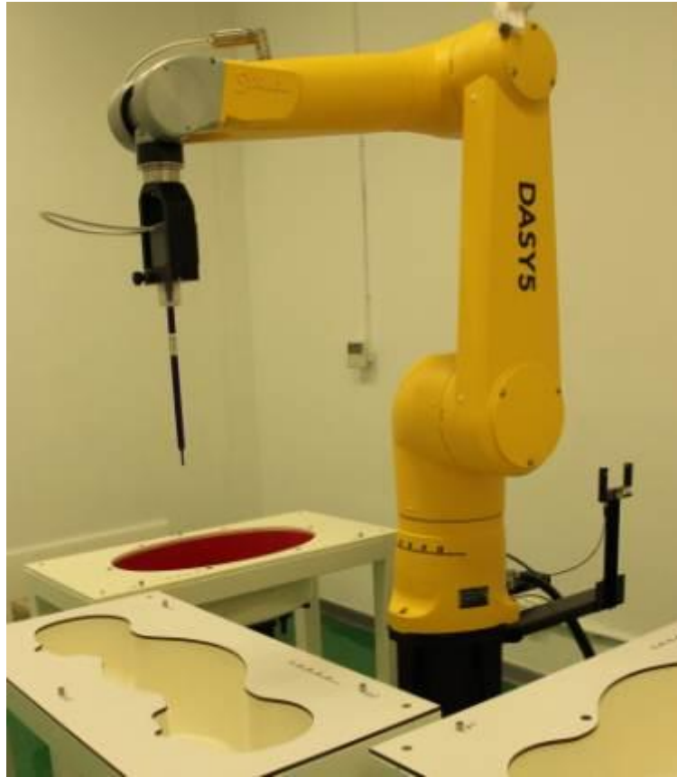
Picture D.3 DSY5 system Set-up
