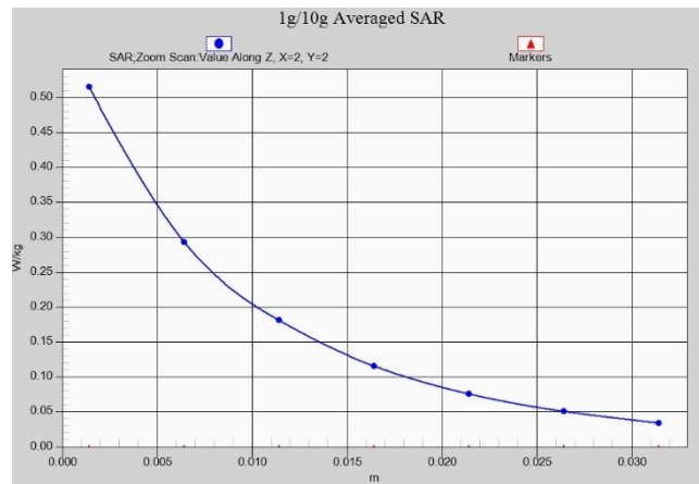
Fig. 1-10 Z-Scan at power reference point (WCDMA850)
