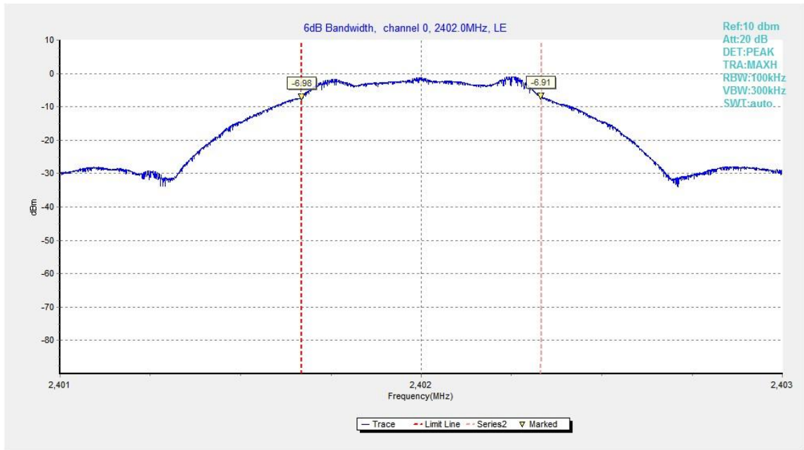
Fig.20. 6dB Bandwidth: GFSK, 2402 MHz
