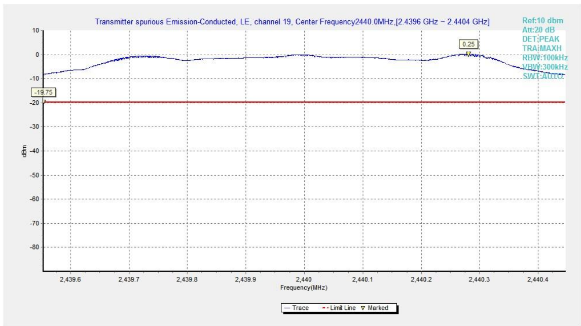
Fig.10. Transmitter Spurious Emission - Conducted: GFSK, 2440MHz
