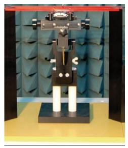
Fig. 2 HAC Phantom & Device Holder
