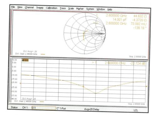
Impedance Measurement Plot for Body TSL
