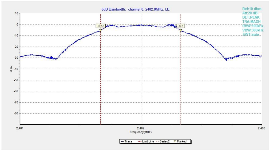
Fig.20. 6dB Bandwidth: GFSK, 2402 MHz
