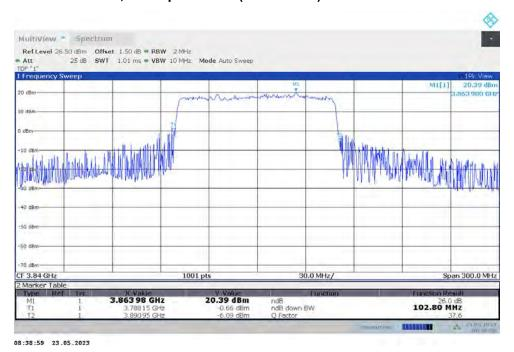
n77H,100MHz Bandwidth,DFT-s-QPSK (-26dBc BW)
