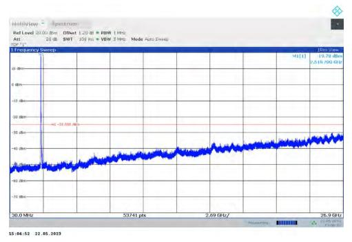
n66 NOTE: peak above the limit line is the carrier frequency.
