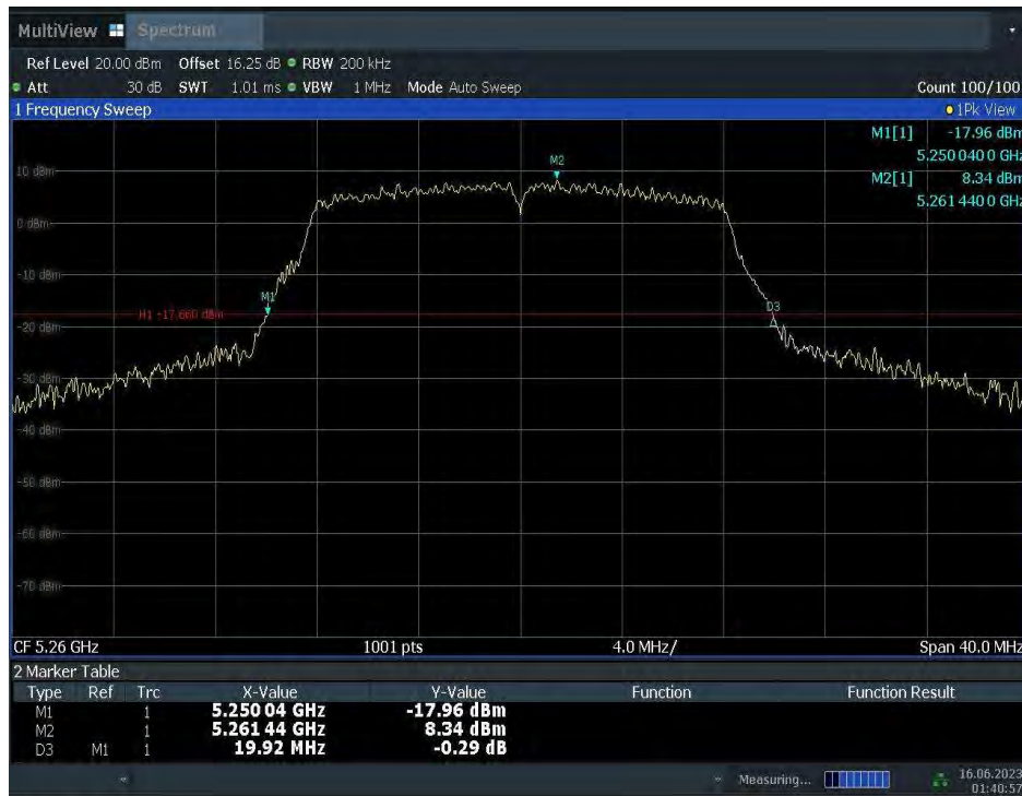
Fig.4 Occupied 26dB Bandwidth (802.11a, 5260MHz)
