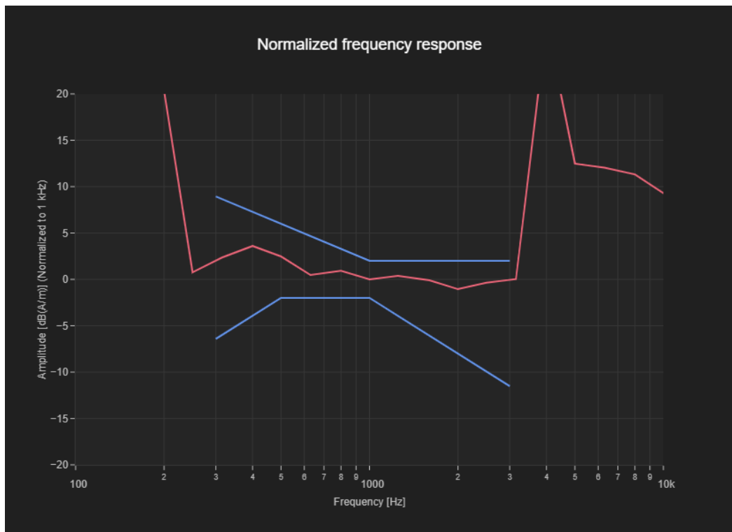
Figure C.4 Frequency Response of NR N78-OTT
