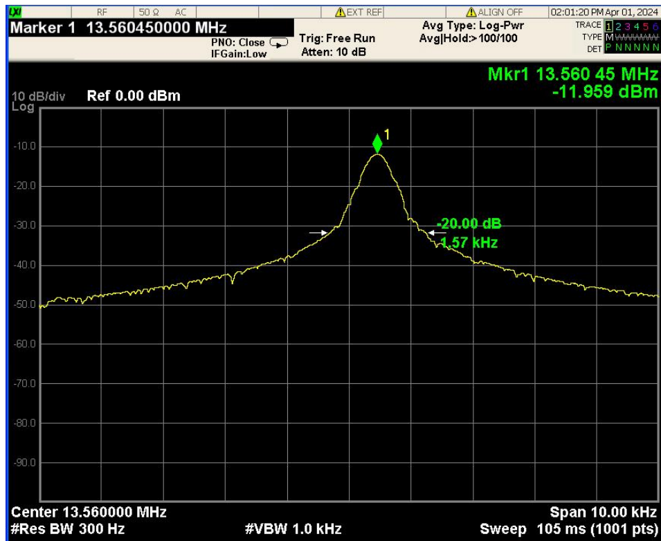
Figure B-9: Measurement results for 20dB Bandwidth
