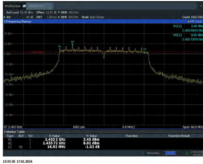
Fig.A.4.9 DTS Bandwidth (802.11n-HT20, Ch 11)
