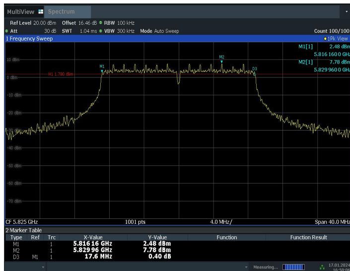
Fig. 6 6dB Emission Bandwidth (802.11n-HT20, Ch 165)
