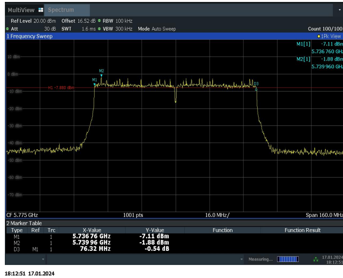
Fig. 9 6dB Emission Bandwidth (802.11ac-VHT80, Ch 155)
