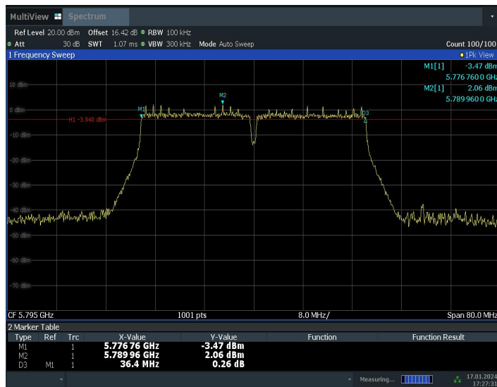
Fig. 8 6dB Emission Bandwidth (802.11n-HT40, Ch 159)
