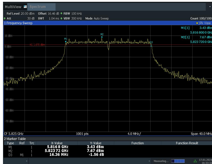
Fig. 3 6dB Emission Bandwidth (802.11a, Ch 165)
