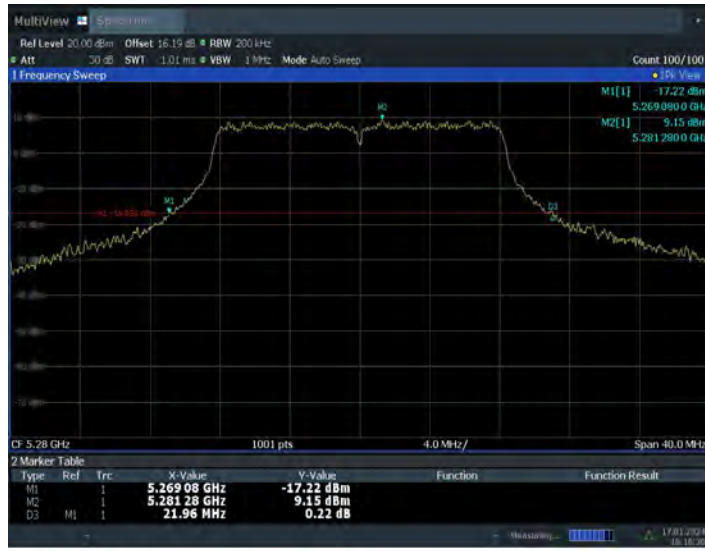
Fig.5 26dB Emission Bandwidth (802.11a, 5280MHz)
