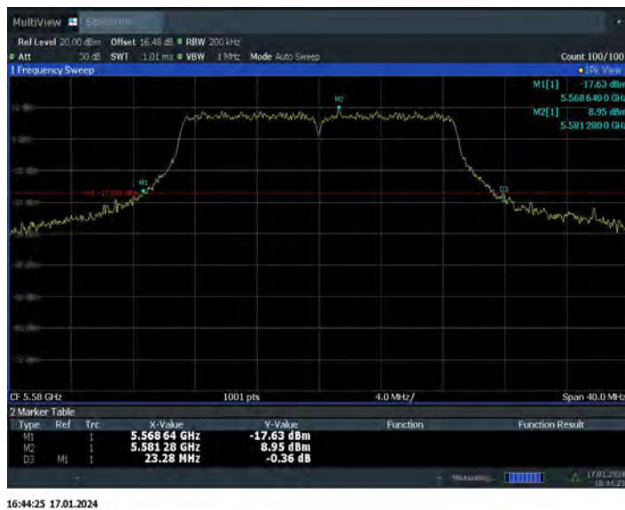
Fig.18 26dB Emission Bandwidth (802. 11n-HT20, 5580MHz)
