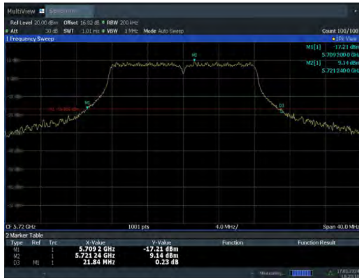
Fig.10 26dB Emission Bandwidth (802.11a, 5720MHz)
