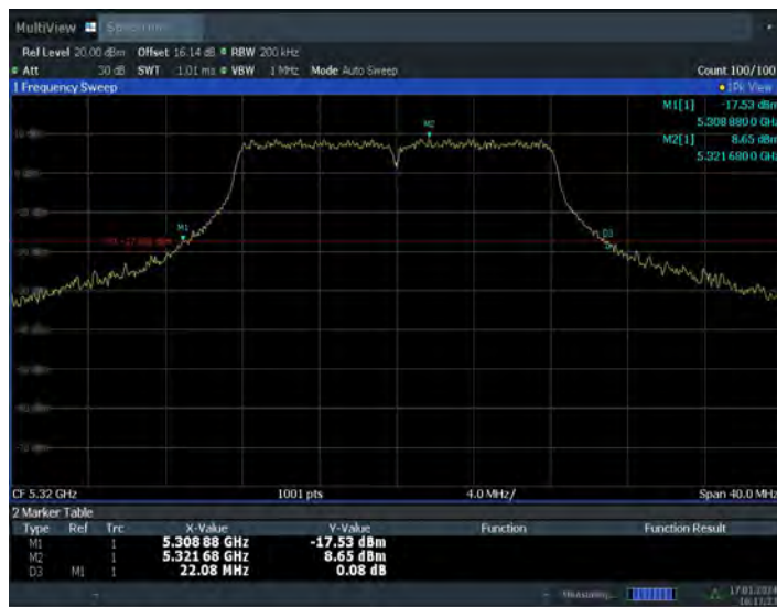
Fig.6 26dB Emission Bandwidth (802.11a, 5320MHz)
