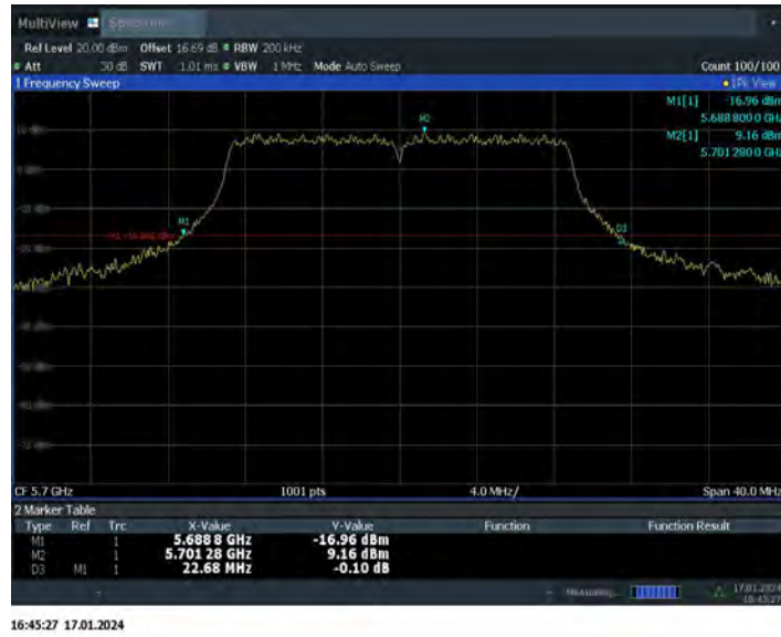
Fig.19 26dB Emission Bandwidth (802. 11n-HT20, 5700MHz)
