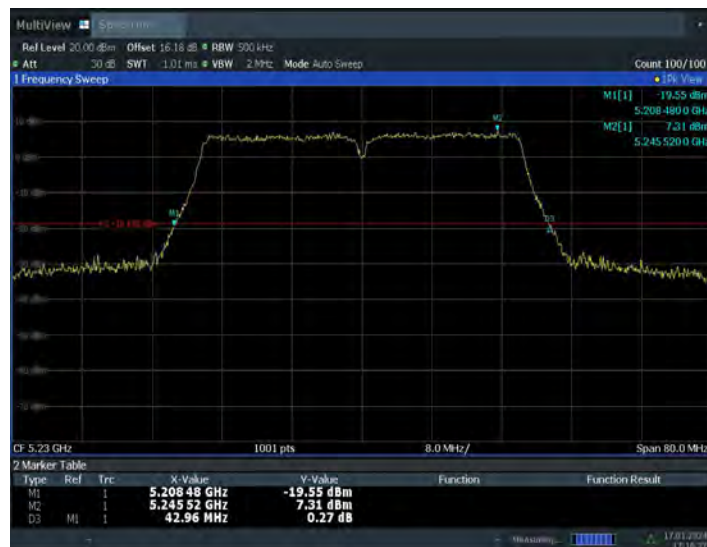
Fig.22 26dB Emission Bandwidth (802.11n-HT40, 5230MHz)
