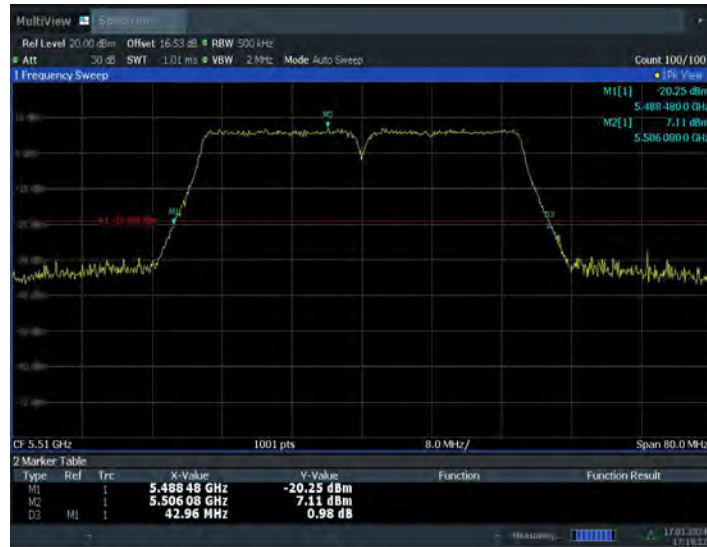
Fig.25 26dB Emission Bandwidth (802. 11n-HT40, 5510MHz)
