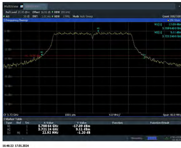
Fig.20 26dB Emission Bandwidth (802. 11n-HT20, 5720MHz)
