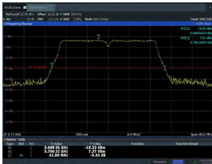
Fig.28 26dB Emission Bandwidth (802. 11n-HT40, 5710MHz)
