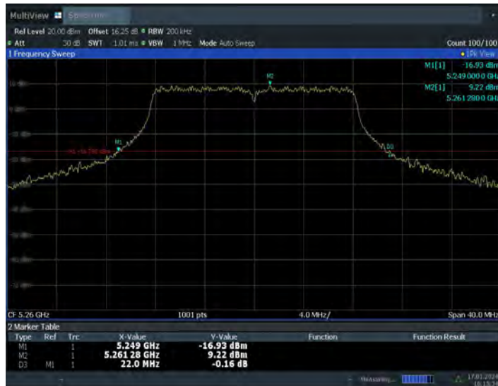
Fig.4 26dB Emission Bandwidth (802.11a, 5260MHz)
