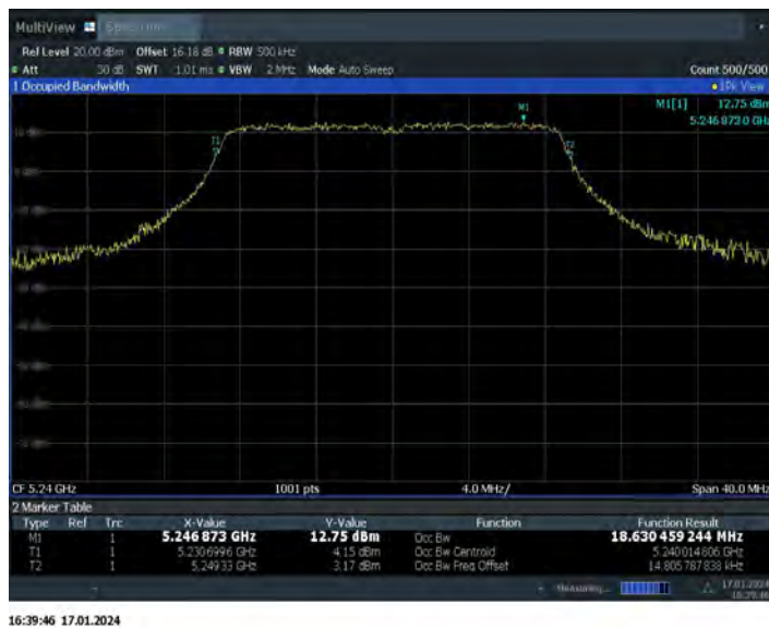
Fig.65 99% Occupied bandwidth (802.11n-HT20, 5240MHz)
