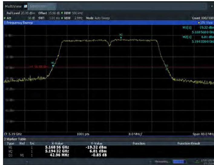
Fig.21 26dB Emission Bandwidth (802.11n-HT40, 5190MHz)
