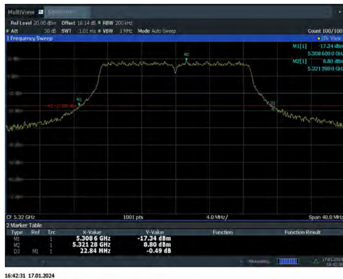
Fig.16 26dB Emission Bandwidth (802.11n-HT20, 5320MHz)
