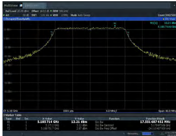
Fig.60 99% Occupied bandwidth (802.11a, 5180MHz)
