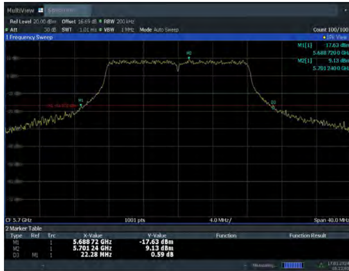
Fig.9 26dB Emission Bandwidth (802.11a, 5700MHz)
