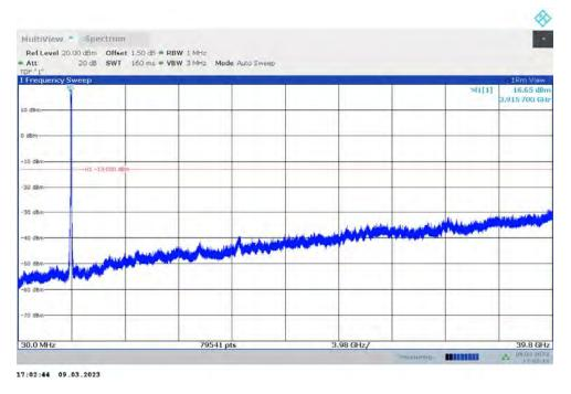
Note: The maximum value of expanded measurement uncertainty for this test item is U = 0.372 dB, k = 2.
