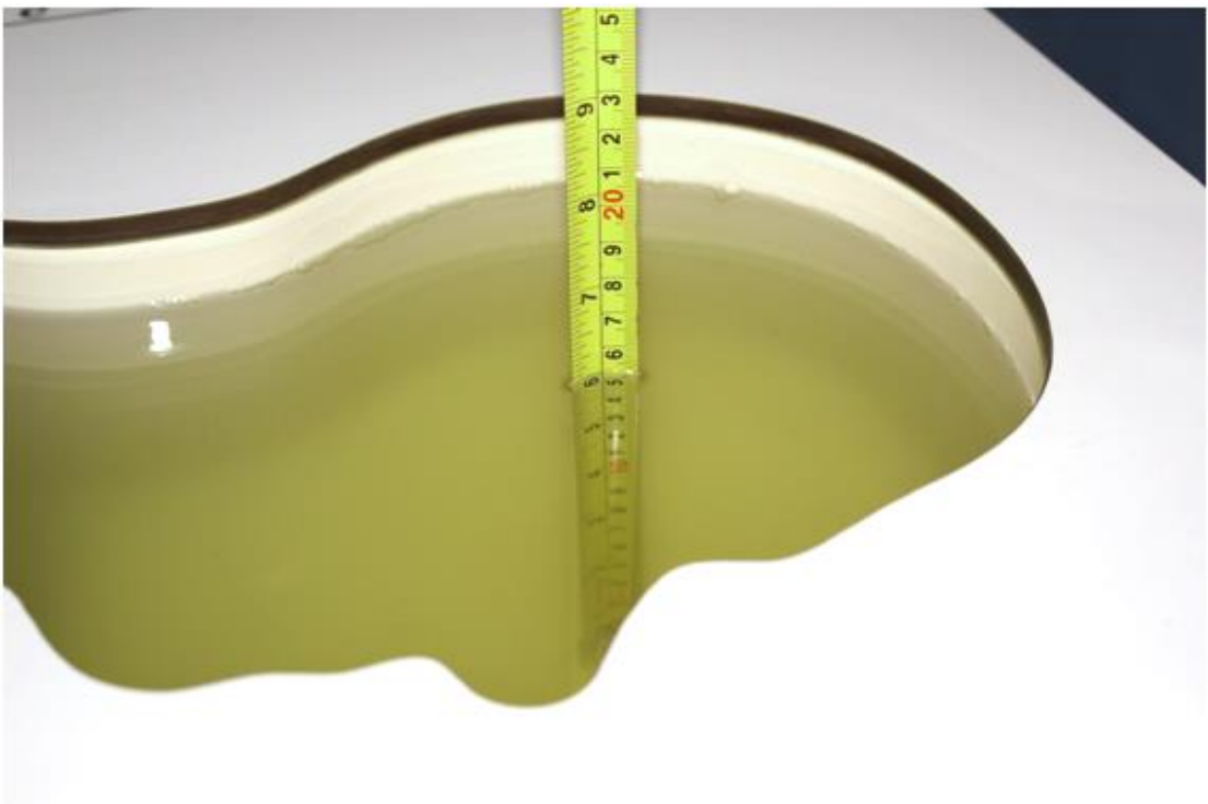
Picture 7-6 Liquid depth in the Head Phantom (2450 MHz)
