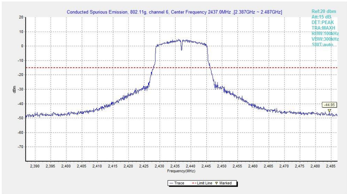
Fig.A.6.1.33 Transmitter Spurious Emission - Conducted (802.11g, Ch6, Center Frequency)
