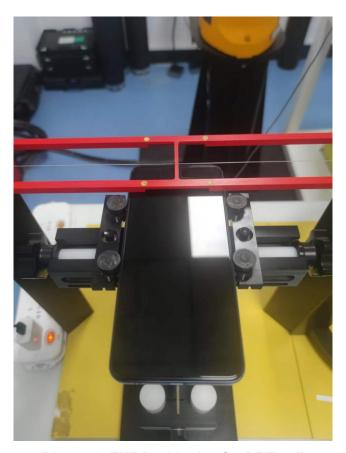
Picture 2: EUT Positioning for RF/T-coil
