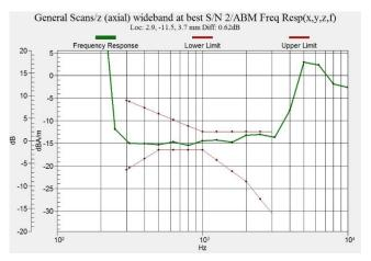
Figure C.2 Frequency Response of GSM850 - OTT VoIP
