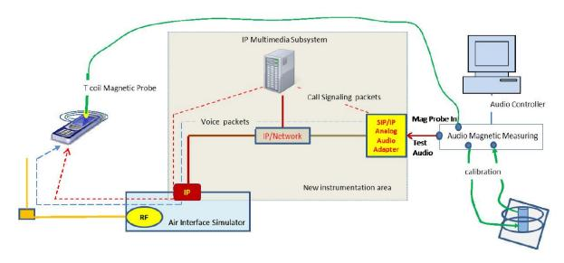
Figure 10.1 Test Setup for VoWiFi over IMS T-coil Measurements
