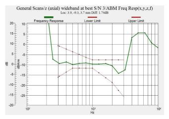
Figure C.1 Frequency Response of GSM850
