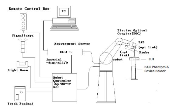
Figure 5.1 HAC Test Measurement Set-up
