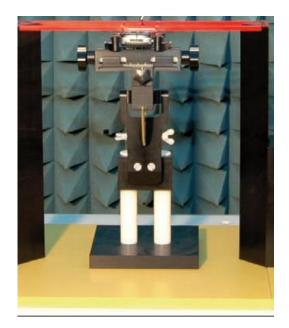
Figure 5.4 HAC Phantom & Device Holder
