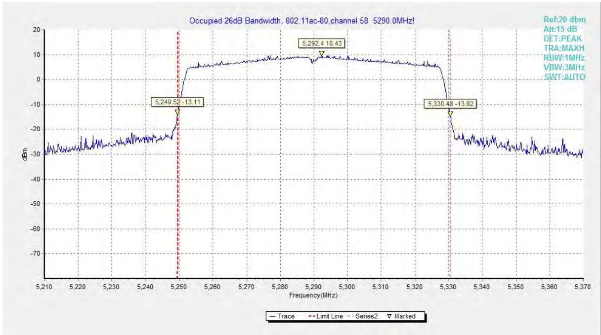
Fig.30 Occupied 26dB Bandwidth (802. 11ac-HT80, 5290MHz)
