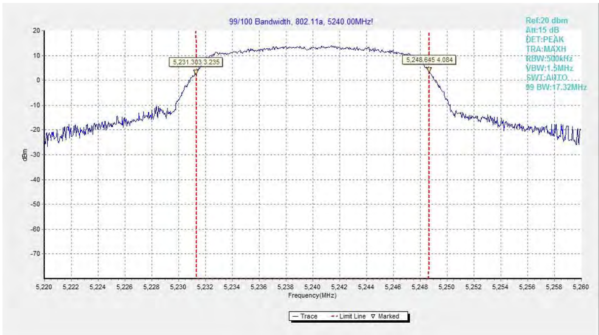
Fig.62 99% Occupied bandwidth (802.11a, 5240MHz)
