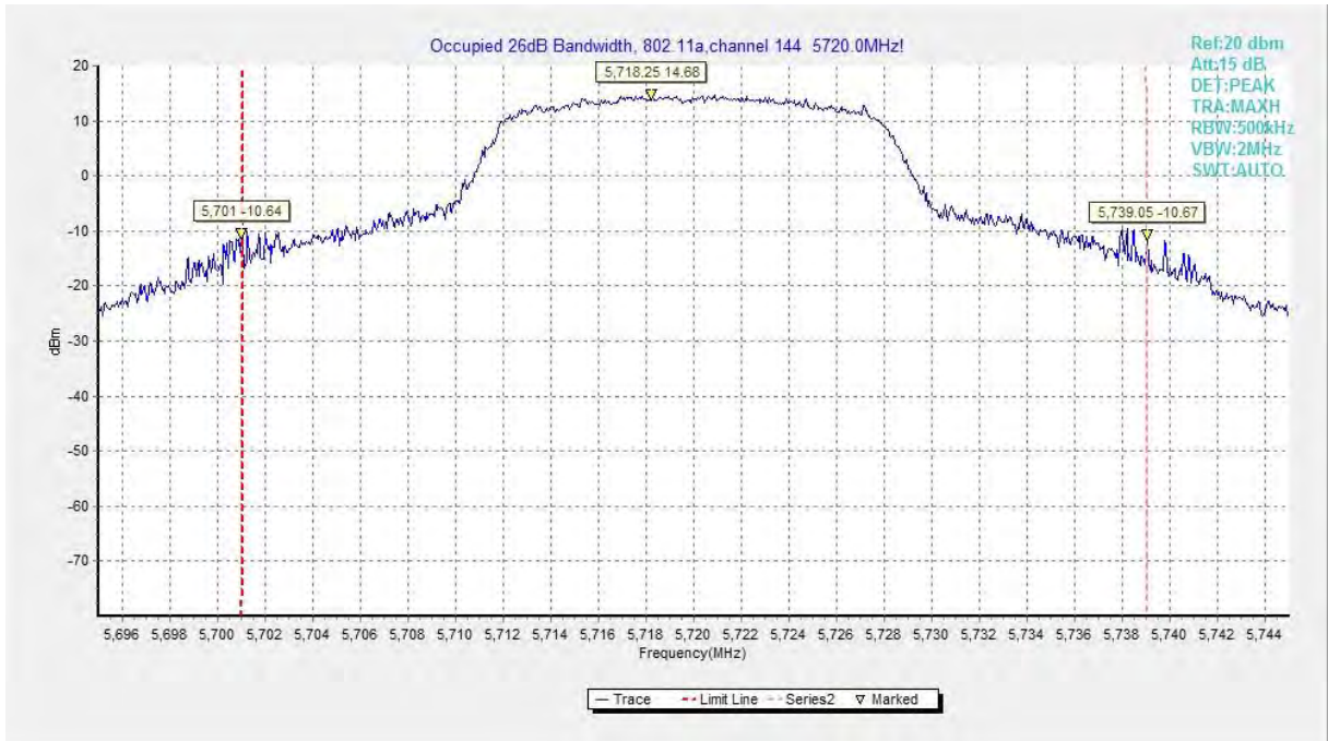
Fig.10 Occupied 26dB Bandwidth (802.11a, 5720MHz)
