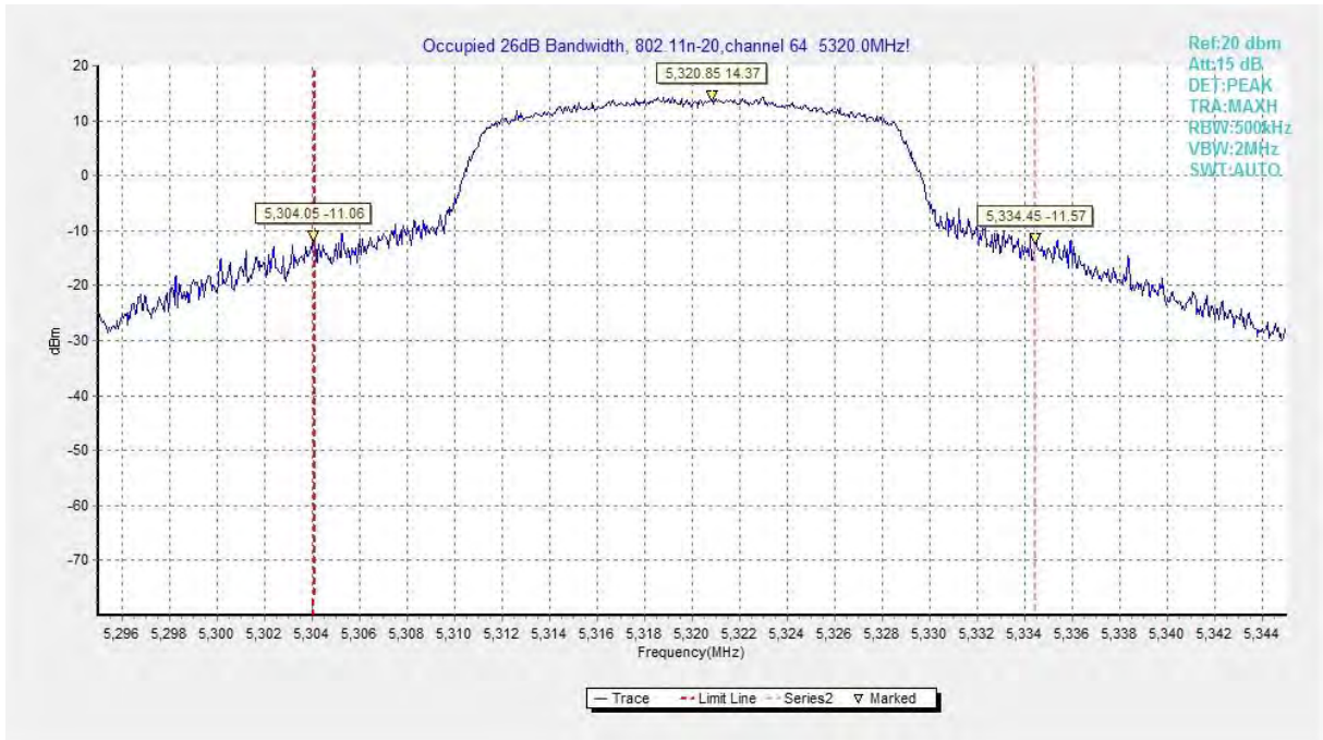
Fig.16 Occupied 26dB Bandwidth (802.11n-HT20, 5320MHz)
