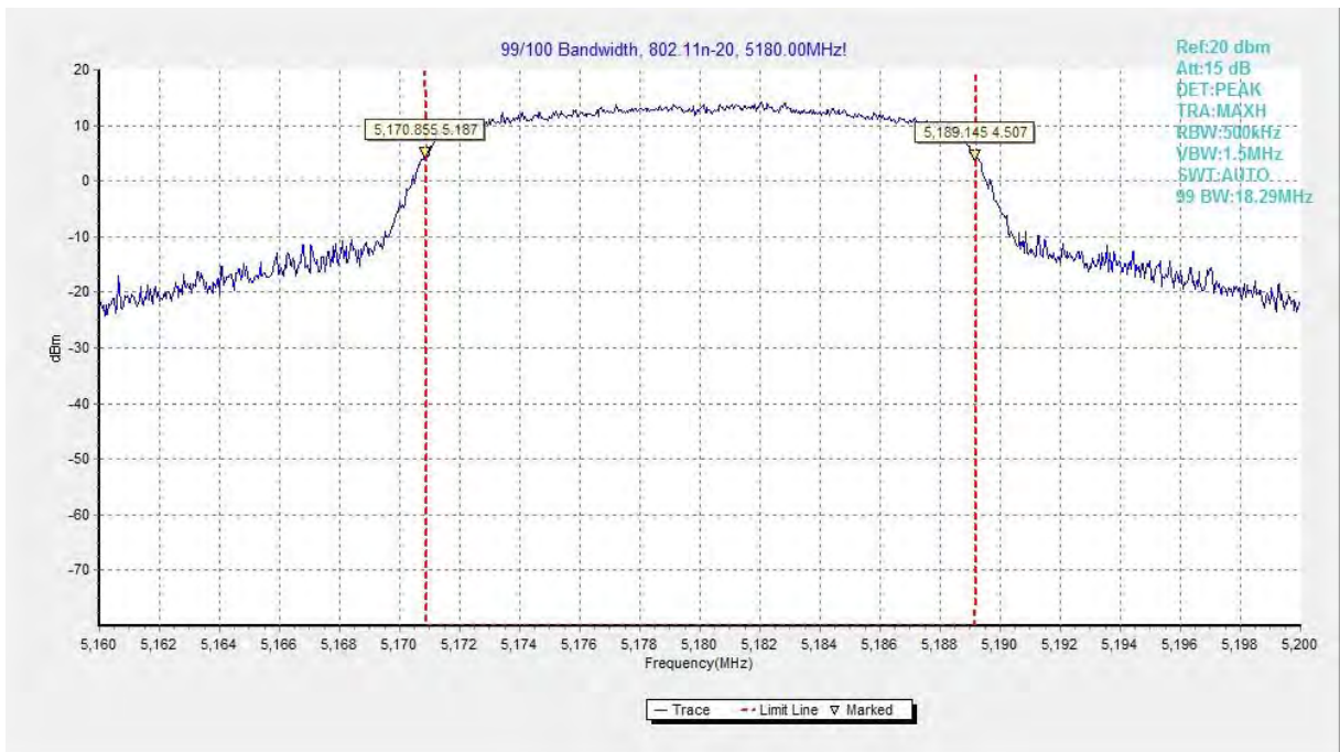
Fig.63 99% Occupied bandwidth (802.11n-HT20, 5180MHz)
