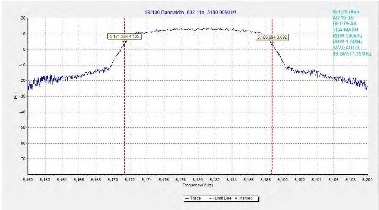
Fig.60 99% Occupied bandwidth (802.11a, 5180MHz)
