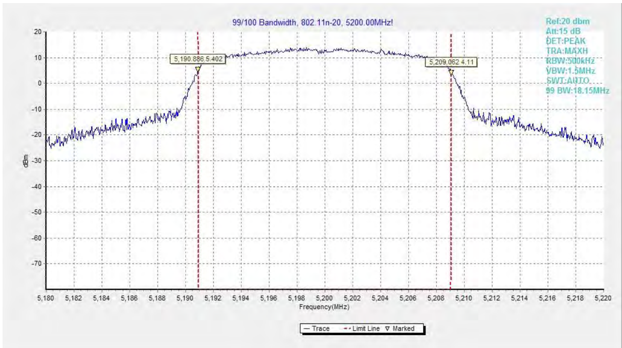
Fig.64 99% Occupied bandwidth (802.11n-HT20, 5200MHz)
