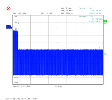
The figure above shows that the client does not transmit any emission within 1800 seconds after getting the order of "stop transmits" from the DFS master (access point).
