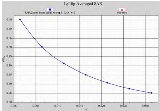
Z-Scan at power reference point (N2 ANT1 Head)
