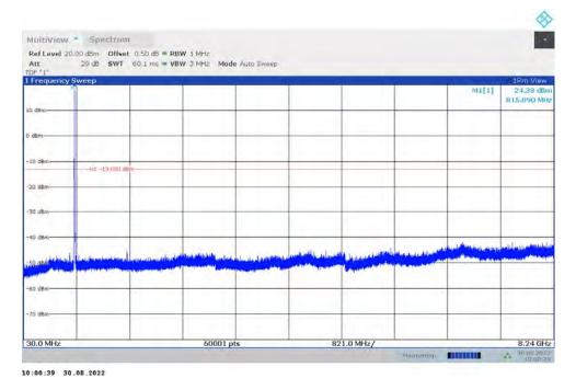
n30 NOTE: peak above the limit line is the carrier frequency.
