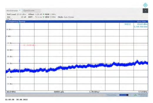
n70 NOTE: peak above the limit line is the carrier frequency.
