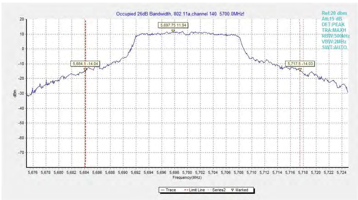
Fig.9 Occupied 26dB Bandwidth (802.11a, 5700MHz)
