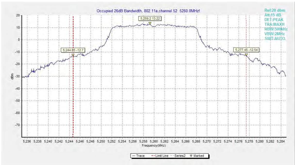
Fig.4 Occupied 26dB Bandwidth (802.11a, 5260MHz)
