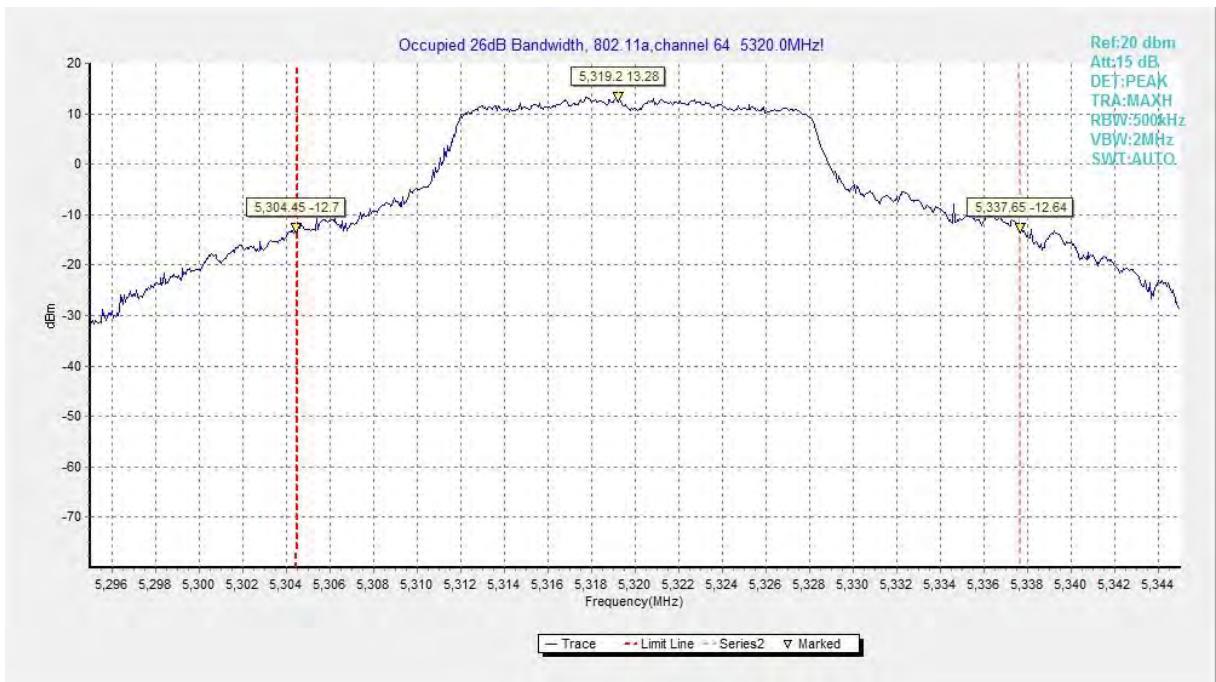
Fig.6 Occupied 26dB Bandwidth (802.11a, 5320MHz)
