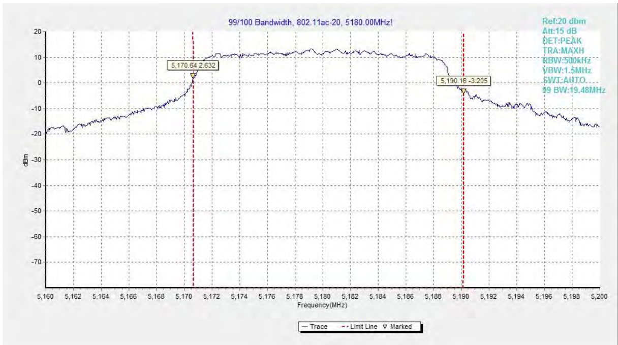
Fig.63 99% Occupied bandwidth (802.11ac-HT20, 5180MHz)
