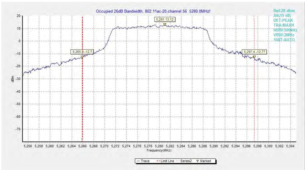
Fig.15 Occupied 26dB Bandwidth (802.11ac-HT20, 5280MHz)
