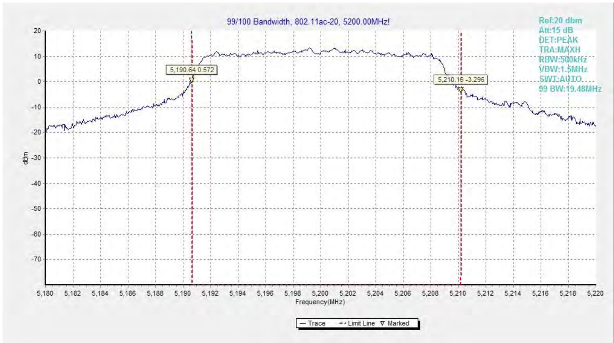
Fig.64 99% Occupied bandwidth (802.11ac-HT20, 5200MHz)
