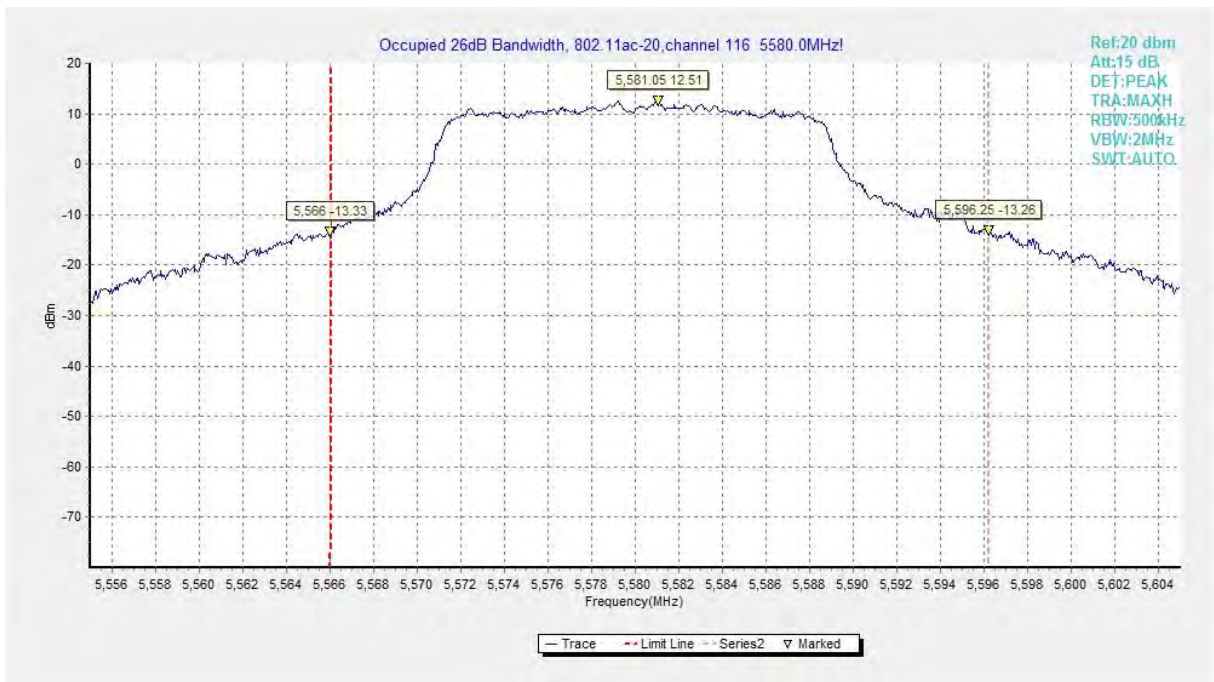
Fig.18 Occupied 26dB Bandwidth (802.11ac-HT20, 5580MHz)
