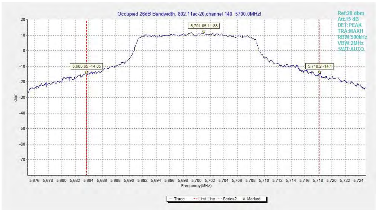
Fig.19 Occupied 26dB Bandwidth (802.11ac-HT20, 5700MHz)
