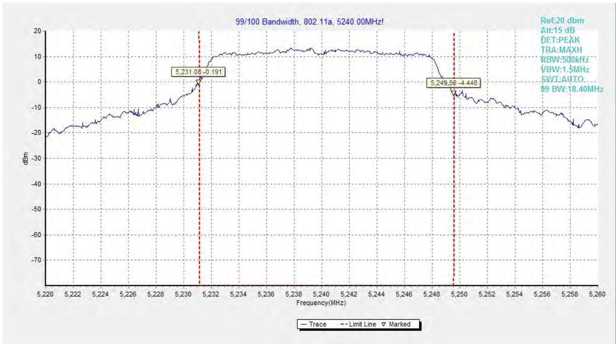
Fig.62 99% Occupied bandwidth (802.11a, 5240MHz)
