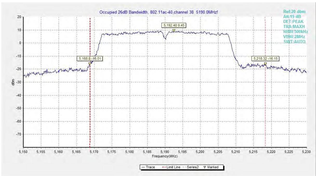
Fig.21 Occupied 26dB Bandwidth (802.11ac-HT40, 5190MHz)
