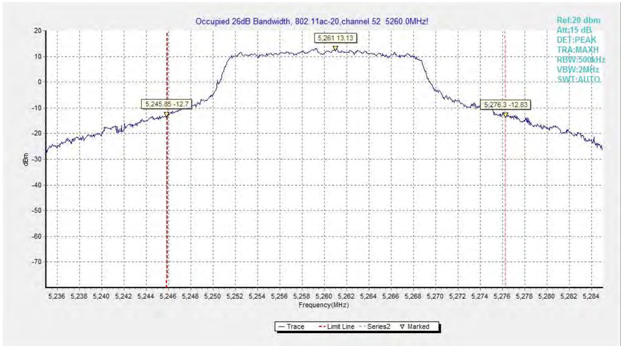
Fig.14 Occupied 26dB Bandwidth (802.11ac-HT20, 5260MHz)
