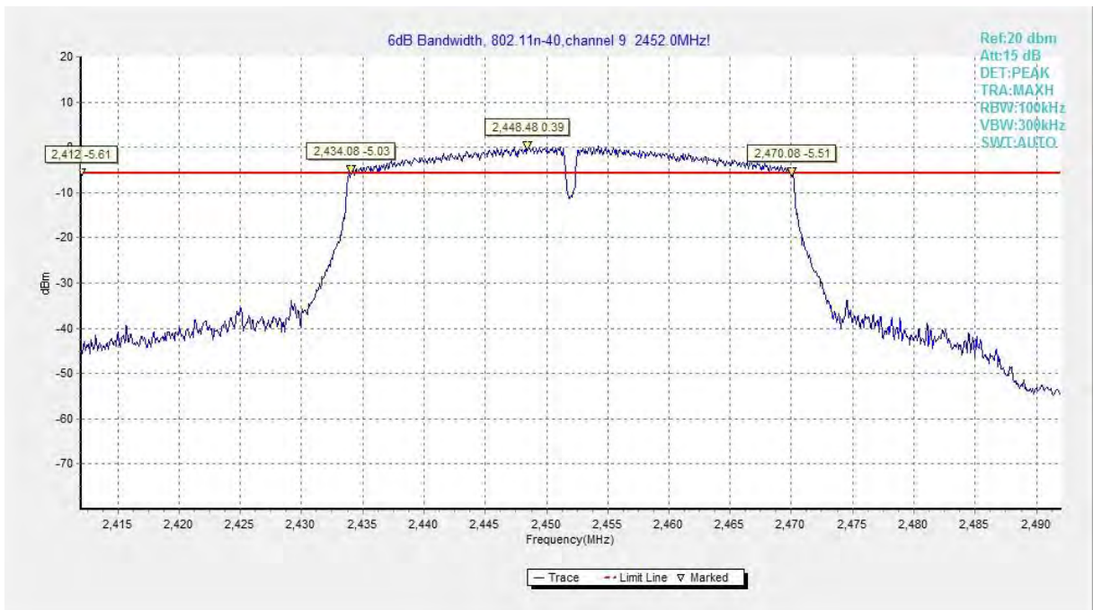
Fig.A.4.12 Occupied 6dB Bandwidth (802.11n-HT40, Ch 9)
