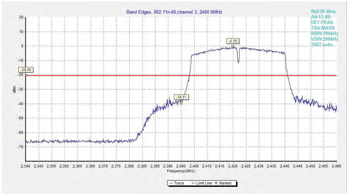
Fig.A.5.7 Band Edges (802.11n-HT40, Ch 3)
