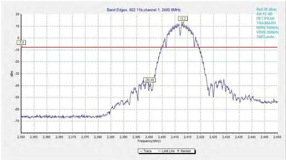
Fig.A.5.1 Band Edges (802.11b, Ch 1)
