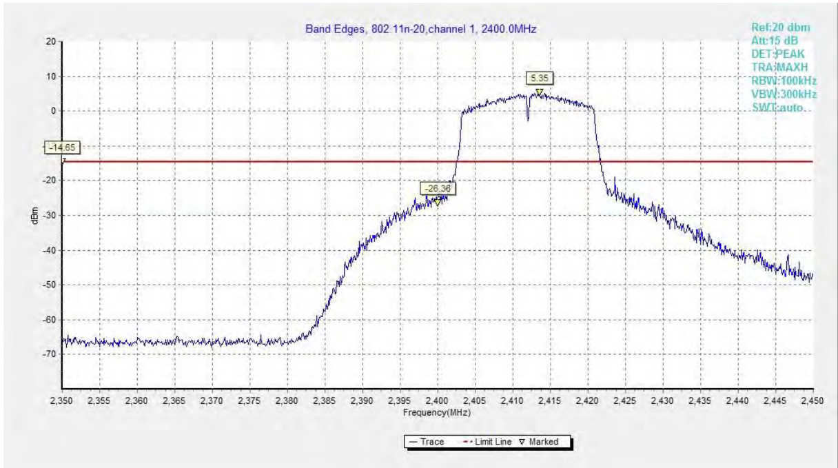
Fig.A.5.5 Band Edges (802.11n-HT20, Ch 1)
