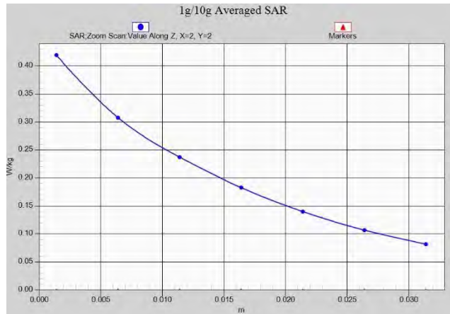
Z-Scan at power reference point (LTE B12 Body)
