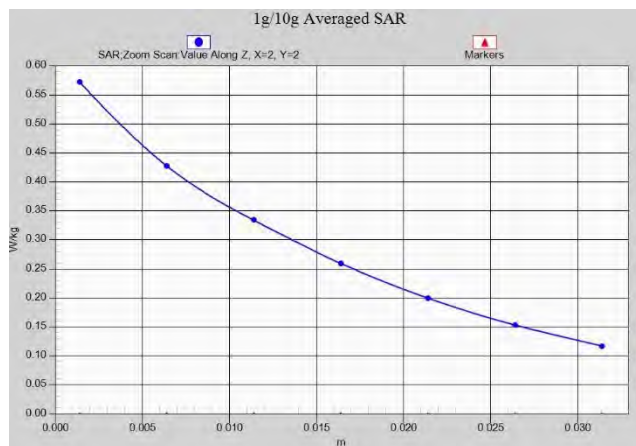
Z-Scan at power reference point (LTE B5 Body)
