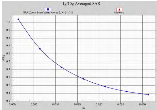
Z-Scan at power reference point (WCDMA1900 MHz Body)
