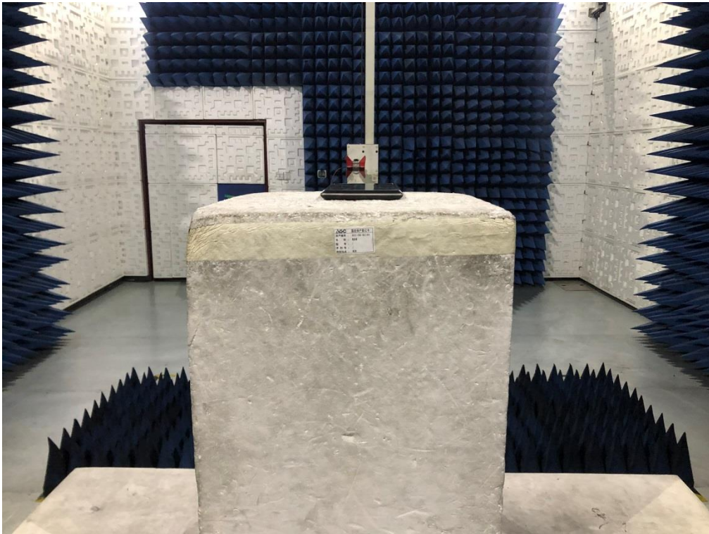
RADIATED EMISSION TEST SETUP ABOVE 1GHZ
