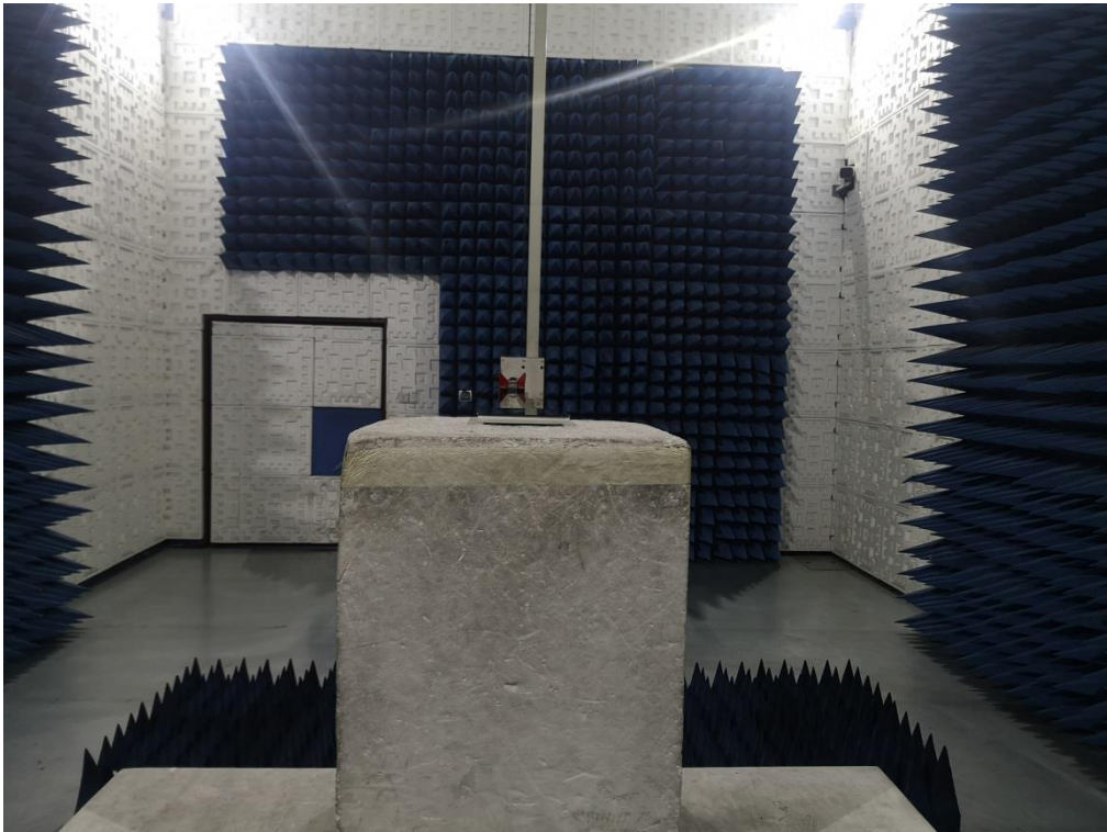
RADIATED EMISSION TEST SETUP ABOVE 1GHZ
