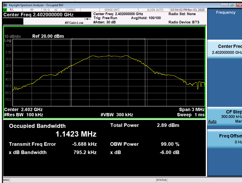
TEST PLOT OF BANDWIDTH FOR LOW CHANNEL
