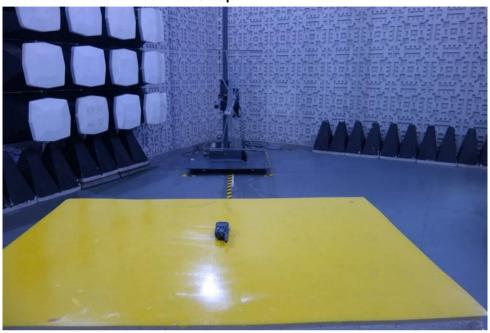
**Radiated Spurious Emissions Test Setup**
