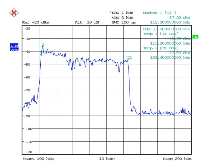
According the test data above, the fundamental wave is not fall in the restricted band 90KHz-110KHz, the field strength also meets the 15.209 requirement, please refer to clause 7.4.
