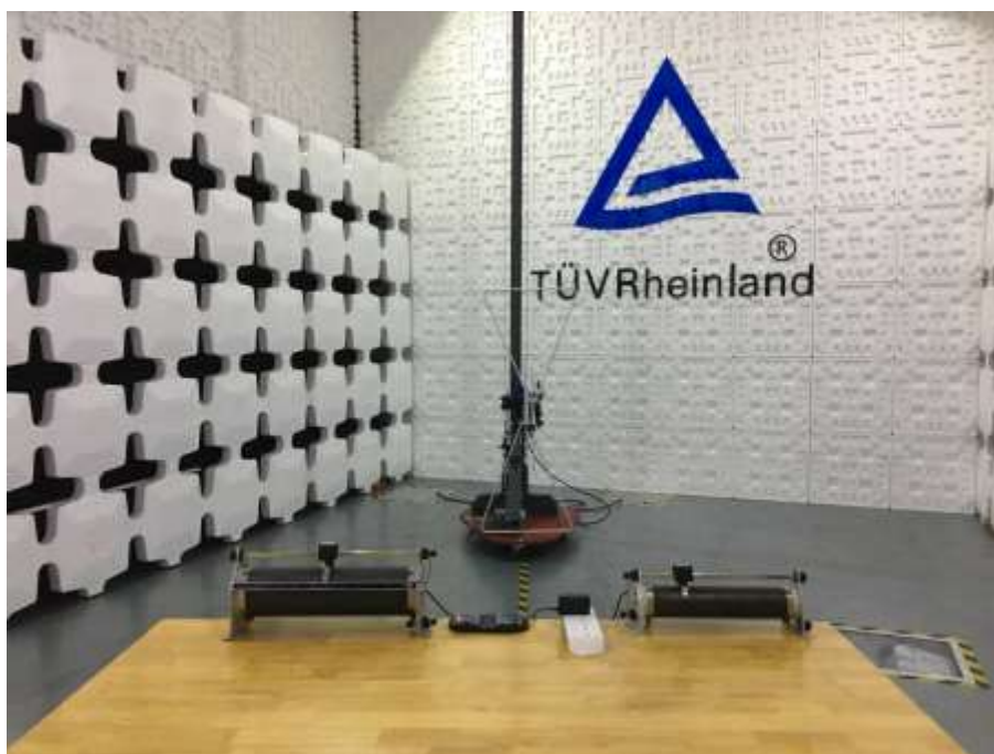
Photograph 2: Set-up photo for Radiated Emission, 30MHz - 1GHz
