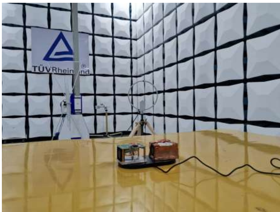
Photograph 1: Set-up photo for Radiated Emission, 9KHz - 30MHz
