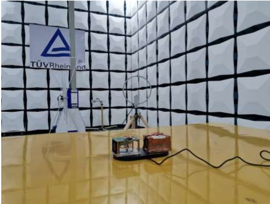
Photograph 1: Set-up photo for Radiated Emission, 9KHz - 30MHz
