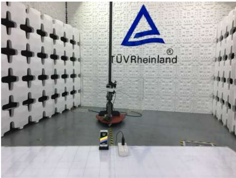
Photograph 2: Set-up photo for Radiated Emission, 30MHz - 1GHz
