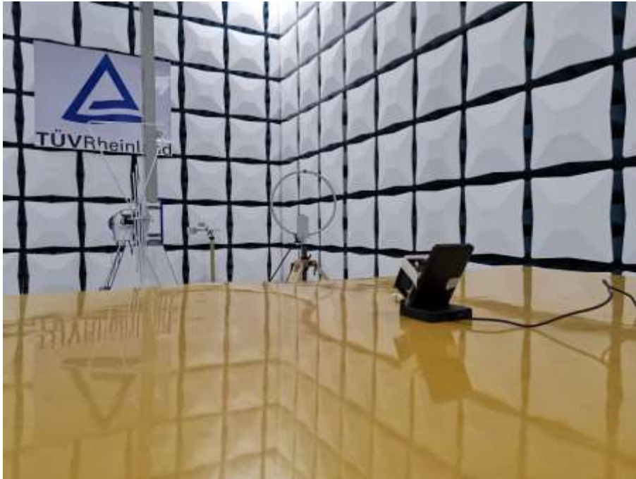
Photograph 1: Set-up photo for Radiated Emission, 9KHz - 30MHz
