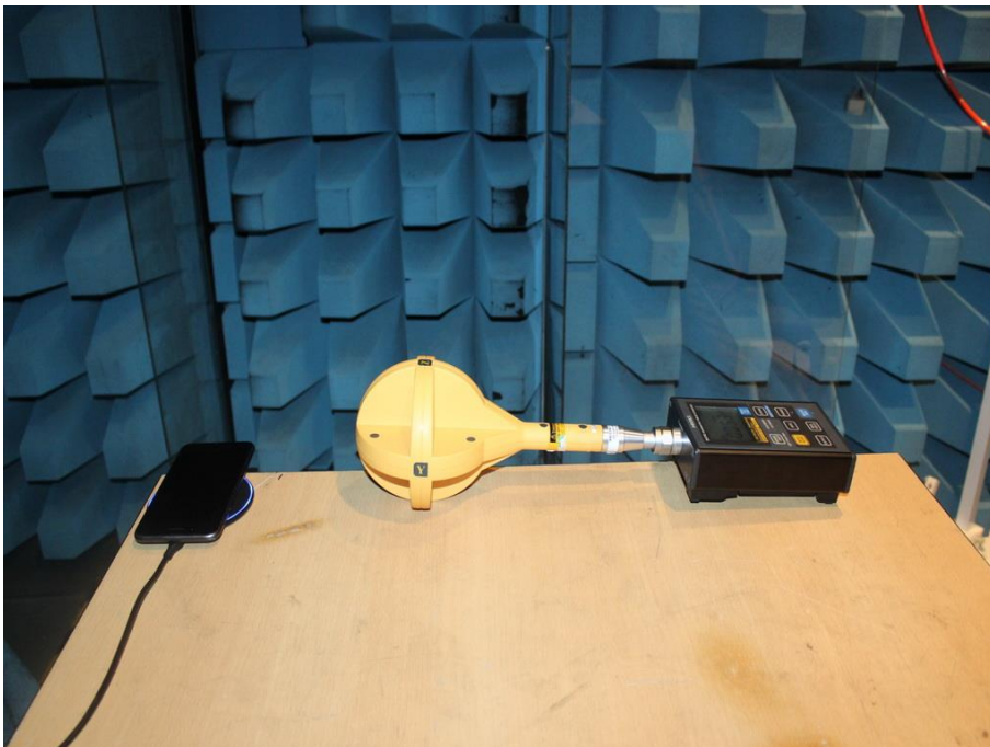
Photograph 4: Set-up for RF Exposure
