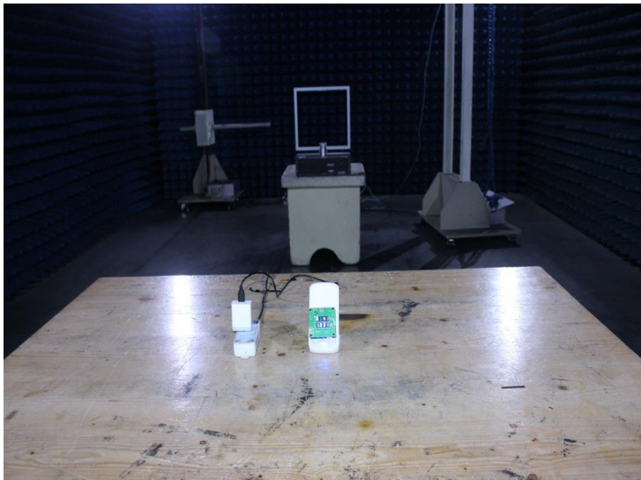
Photograph 2: Set-up for Radiated Spurious Emission, 30MHz - 1GHz
