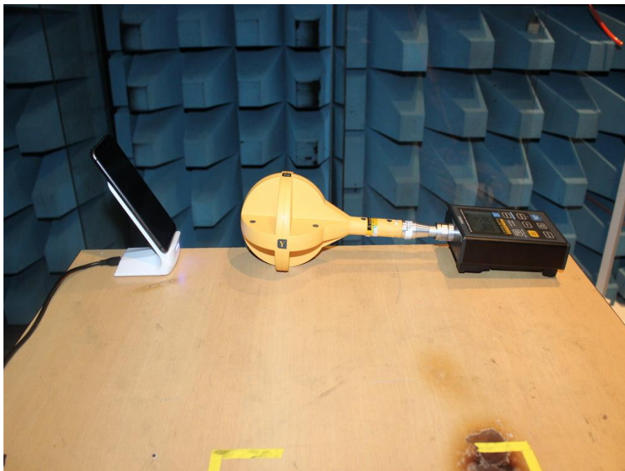
Photograph 4: Set-up for RF Exposure
