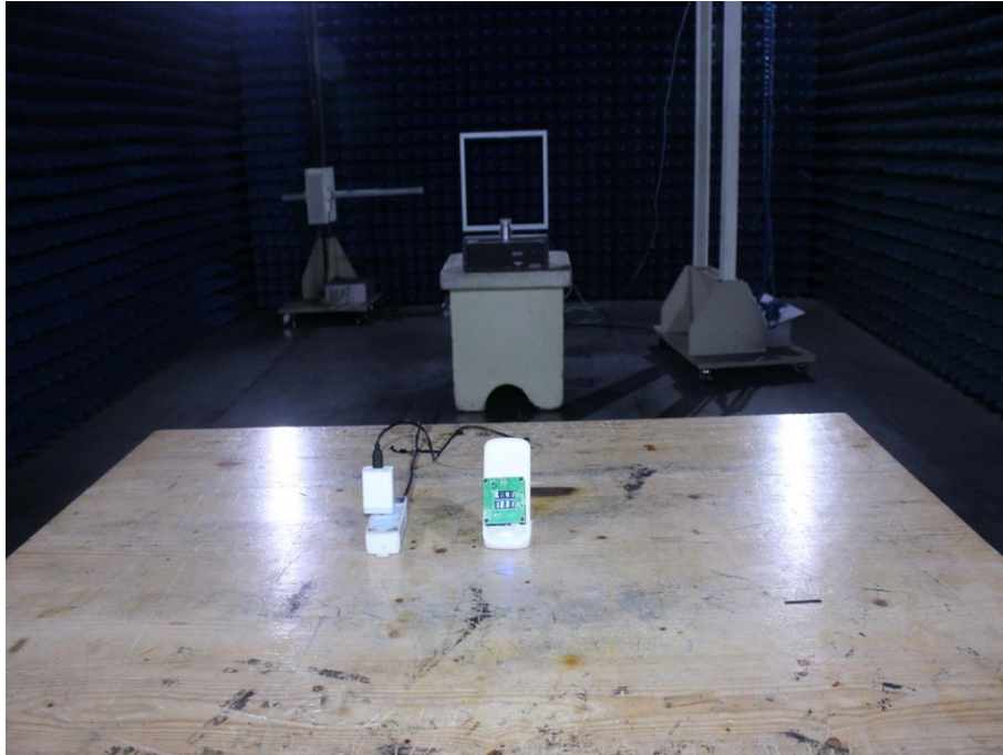
Photograph 1: Set-up for Radiated Spurious Emission, 9KHz - 30MHz
