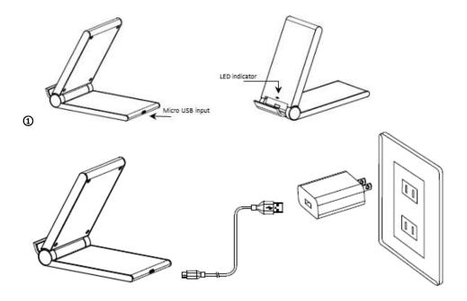
1, Insert the USB end of cable into power adaptor, and connect Micro-USB end of the cable with the wireless charger, the green LED indicator lights up after it is connected well.
