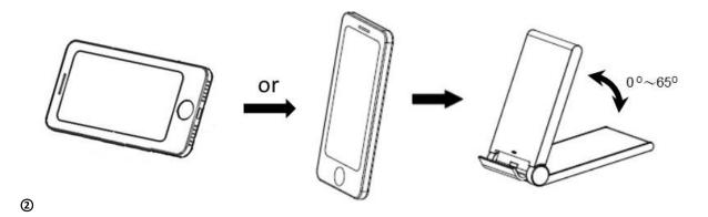
2, Put your mobile phone vertically or horizontally on the wireless charging stand and ensure its center aligns with the center of wireless charger. Besides, you can adjust your wireless charging stand angle from 0 to 65 degree you want while using.
