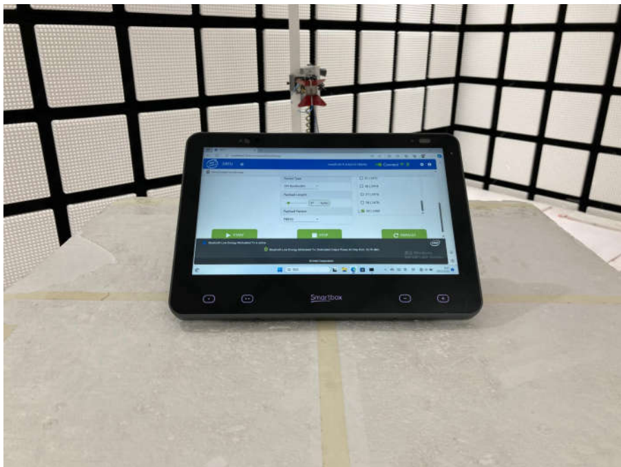
Radiated spurious emission Test Setup-3(Above 1GHz)
