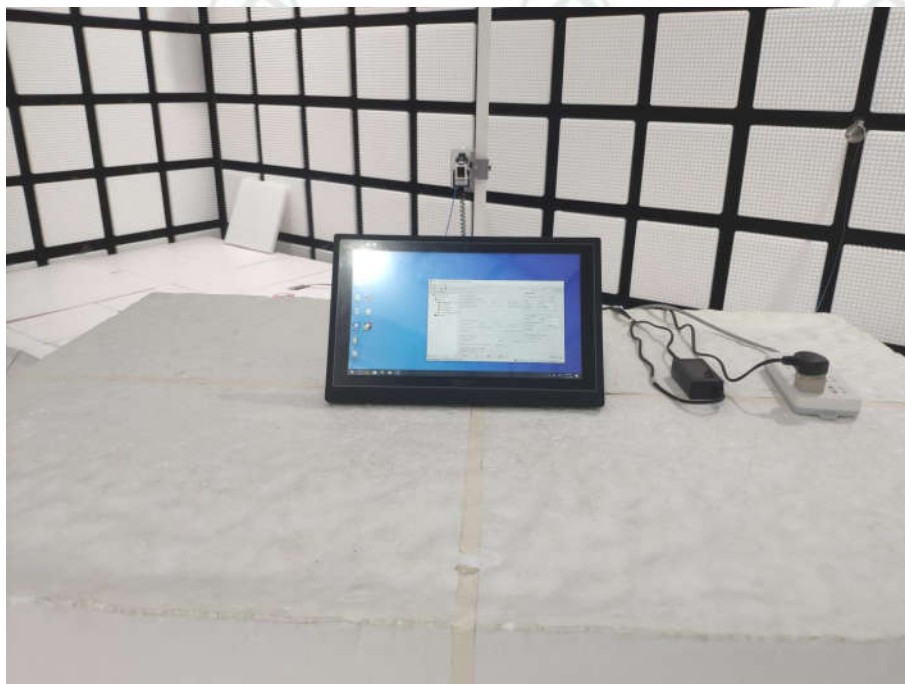
Radiated spurious emission Test Setup-5(Above 18GHz)
